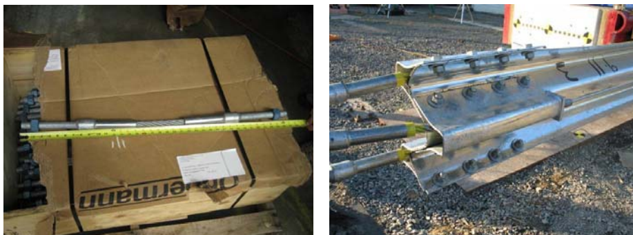
Figure 20. Custom Swaged Anchor Cable (left) and W-Beam Rail End Anchorage Assembly (right)
