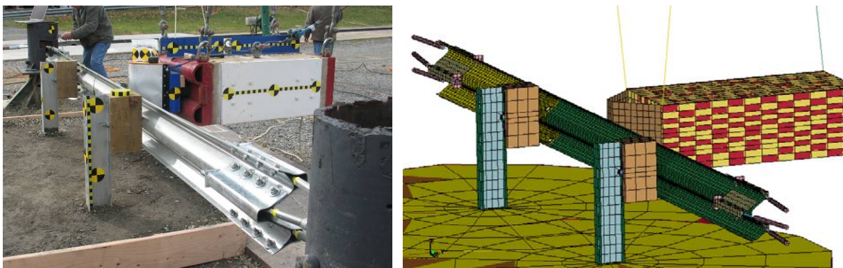
Figure 28. Undamaged Strong Post W-Beam Barrier Test Setup
