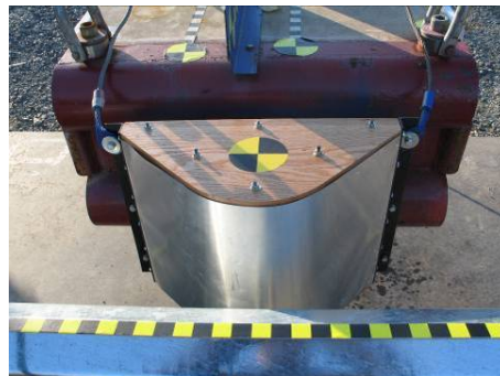
Figure 23. Triangular Impactor Face Mounted to the 2000-kg FOIL Pendulum
