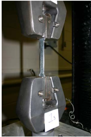
Figure 62. Quasi-Static Tensile Testing Setup
