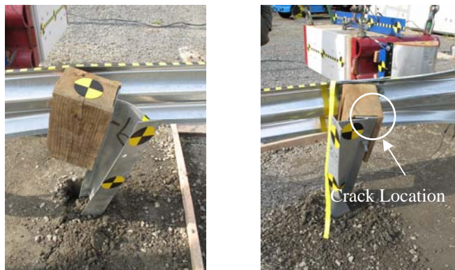
Figure 25. Post Damage at Non-Splice Location (left) and Splice Location (right)
