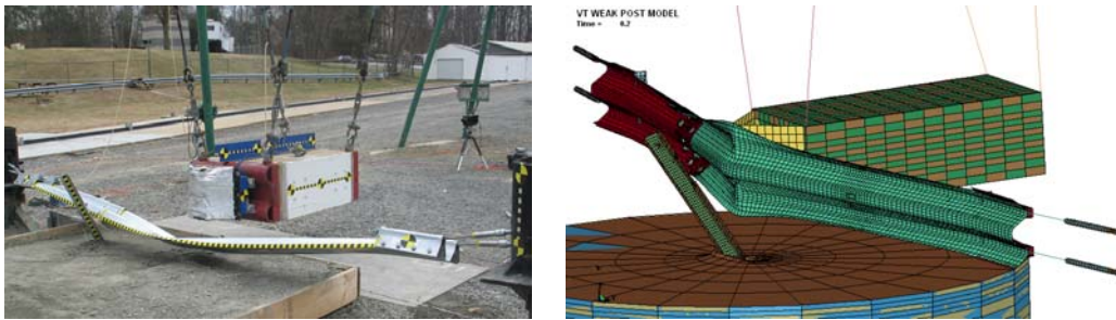
Figure 49. Post Impact Images of Test and Simulation of the Test Level 2 Weak Post Barrier
