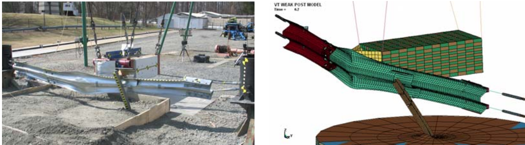
Figure 51. Post Impact Images of Test and Simulation of the Test Level 3 Weak Post Barrier
