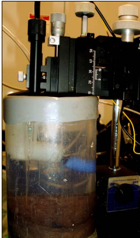
Figure 5. Laboratory sediment core microprofiling setup.
