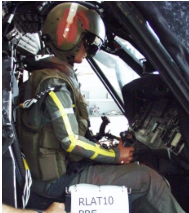
Figure F9: Test setup with dummy dressed in flight suit and situated in typical aviator position.
