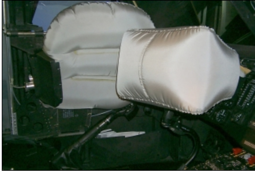
Figure F6: Copilot forward and side airbags under static inflation in a flight simulator.
