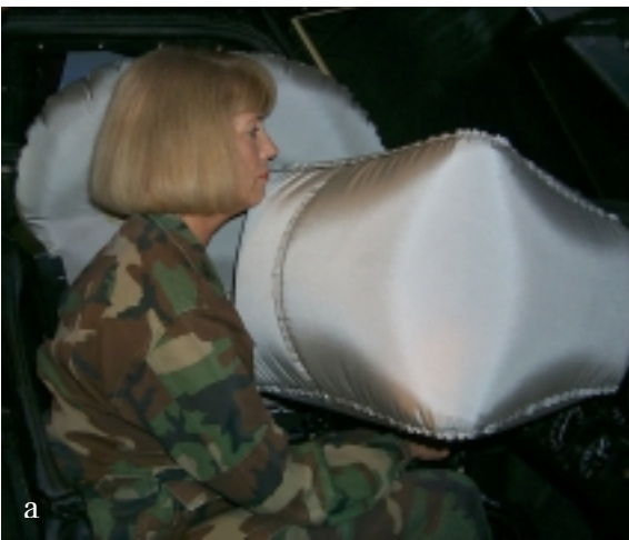
Figure F13: Comparison of female (a) and male (b) aviator stature positions in relation to airbag deployments.
