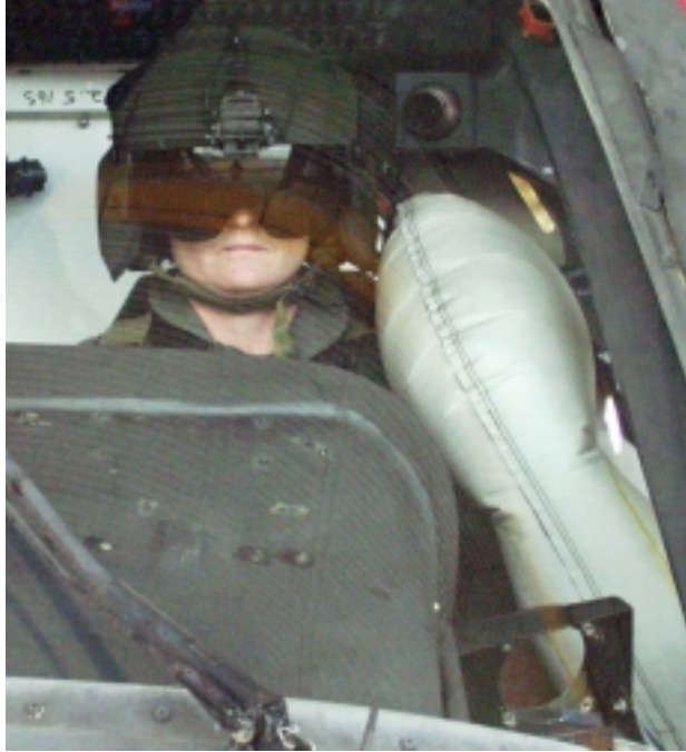
Figure F8: Enhanced side airbag viewed from the nose of the aircraft.
