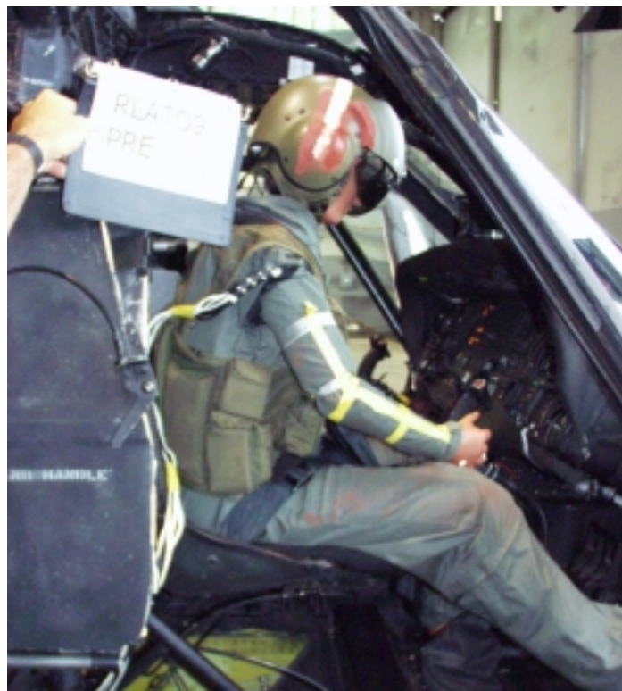
Figure F11: Dummy's seat positioned to represent typical aviator position.
