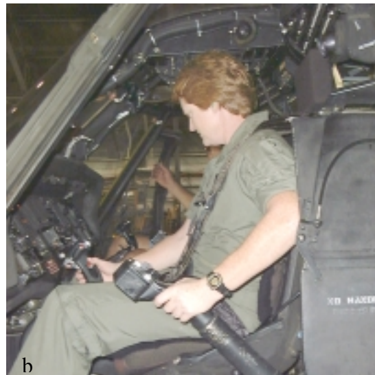
Figure F12: Comparison of dummy worst case position (a) and stature of 2 nd percentile female aviator (b).
