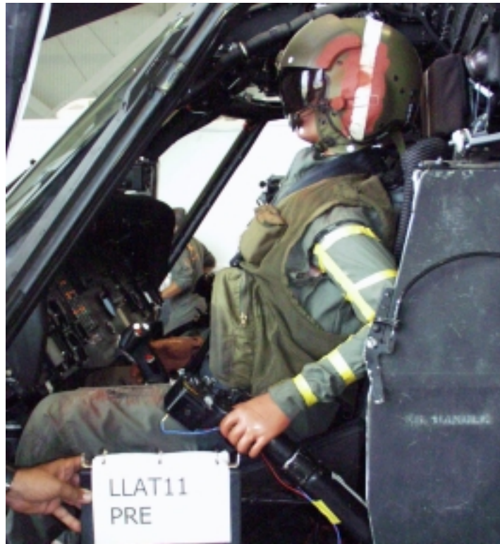
Figure F10: Dummy's seat positioned to represent a worst case scenario.
