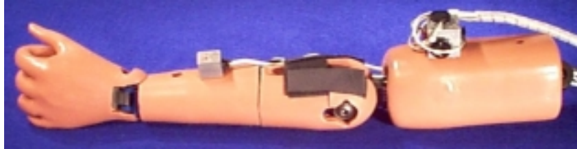
Figure F1: SAE 5 th percentile female instrumented upper extremity (Denton ATD, Inc.).
