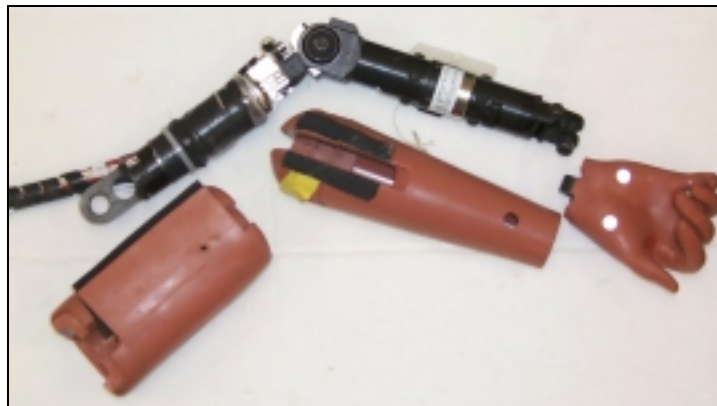
Figure F2: SAE 5 th percentile female instrumented upper extremity disassembled (Denton ATD, Inc.).
