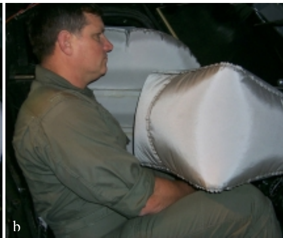
Figure F13: Comparison of female (a) and male (b) aviator stature positions in relation to airbag deployments.
