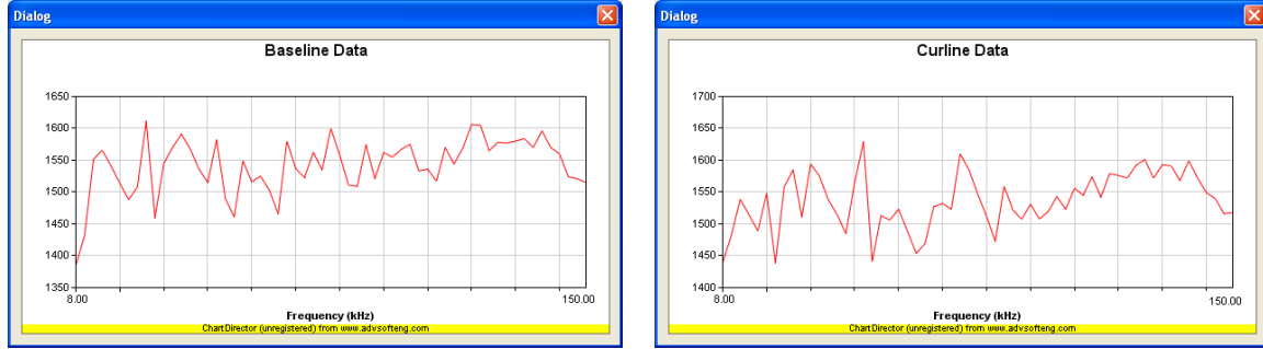
(a) Healthy structure (b) Damaged structure Figure 2-8. Phase profiles of the healthy and damaged structures
