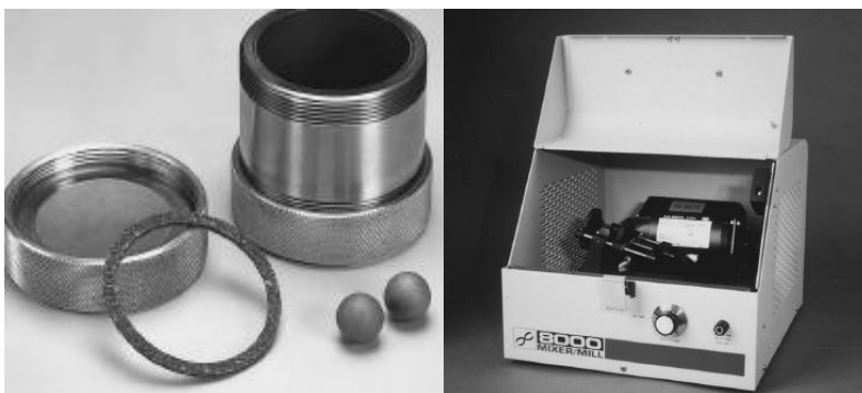
Figure 11 WC milling vial and balls on left and SPEX 8000 mill on right [35] Reprinted with permission from Elsevier.
