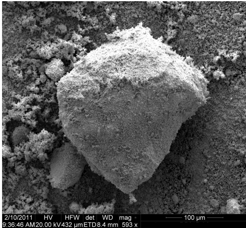
Fig. A2.10 SEM micrograph of 100 hour milled W-3Ni-1Fe particles
