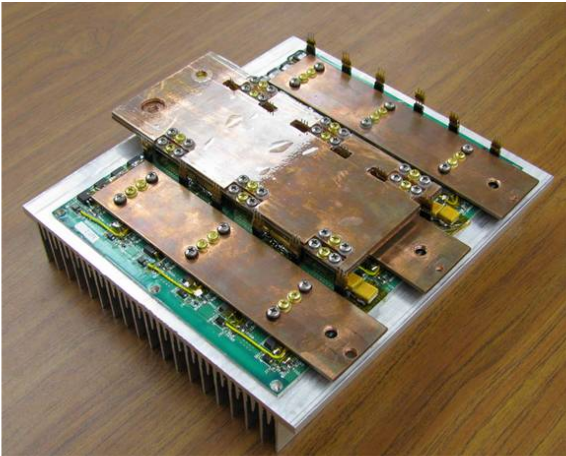
Figure 4.5 – Picture of half-bridge converter bus bar configuration
