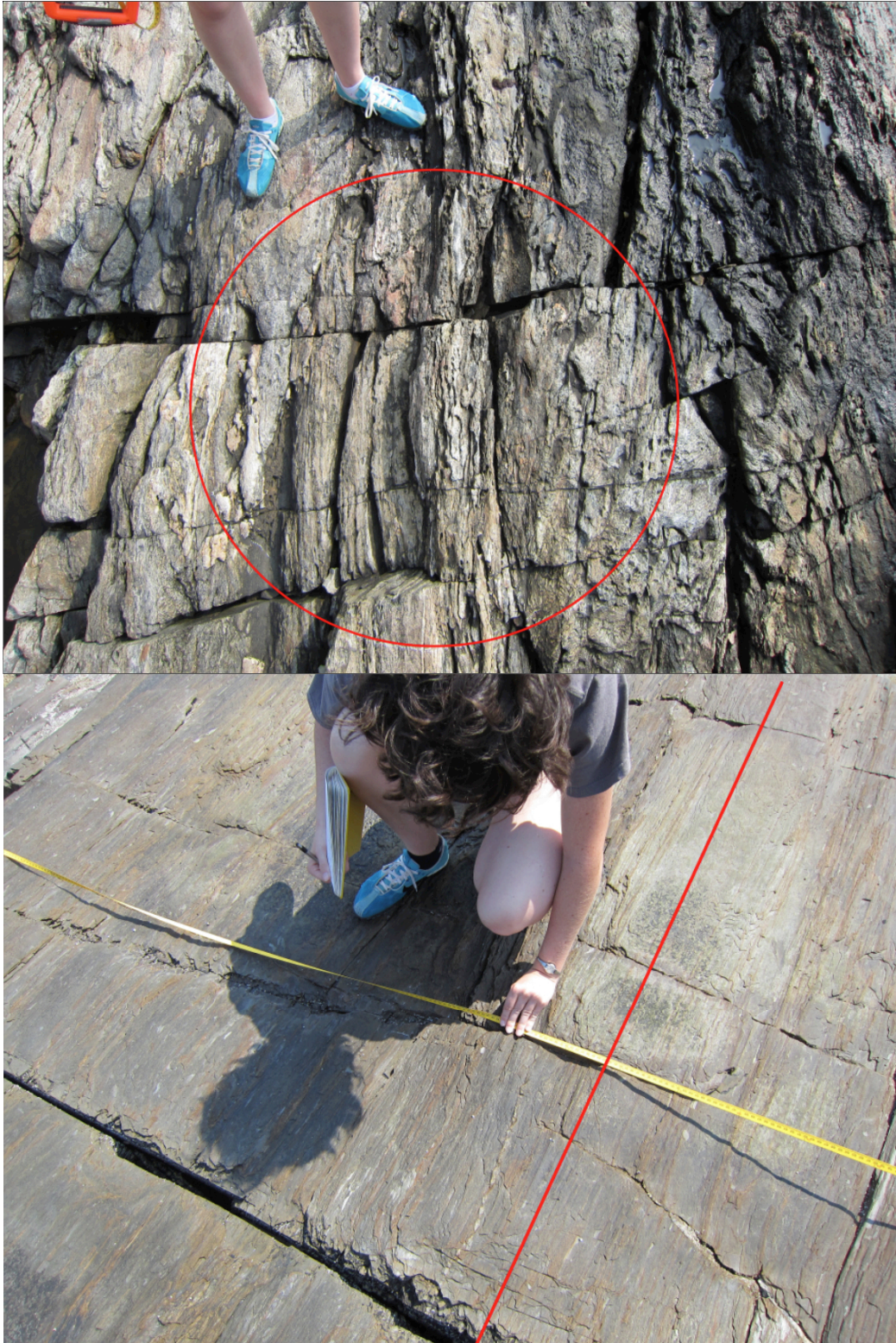
Figure 2d Top: example of a circular window (110 cm diameter) with red circle highlighting the drawn chalk line. Several of these were used at each outcrop. Bottom: example of intersecting scanlines, with red line representing the orientation of a second scanline.
