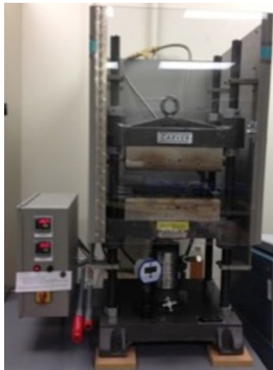
Figure 3.7 Carver hot press for pressure assisted sintering of nanosilver paste.
