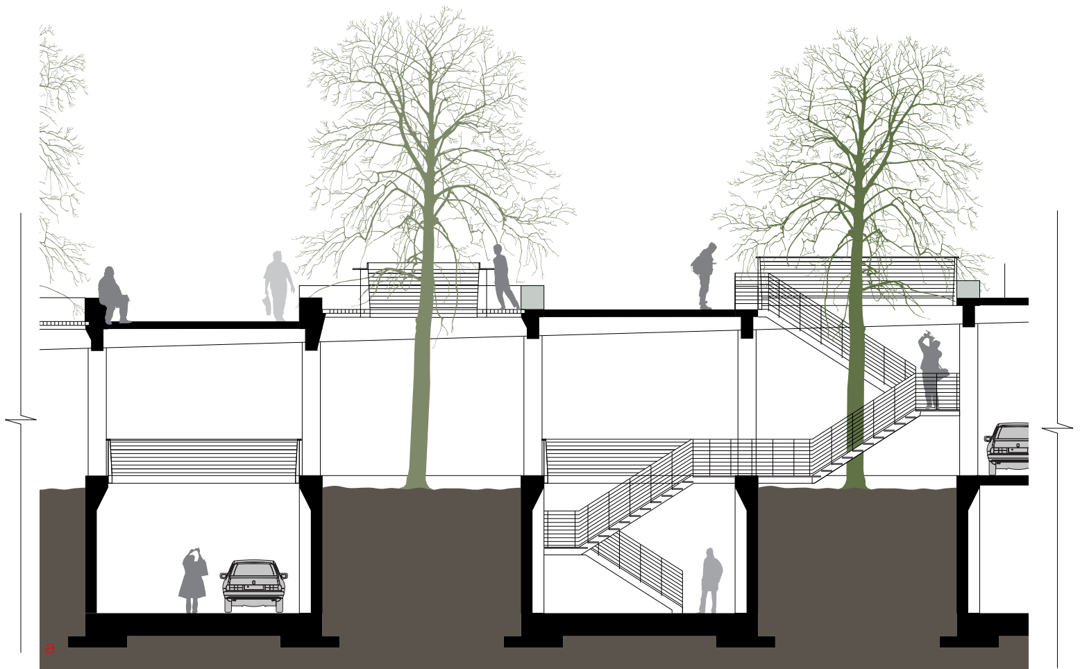
Section- through stairwells and tree boxes
