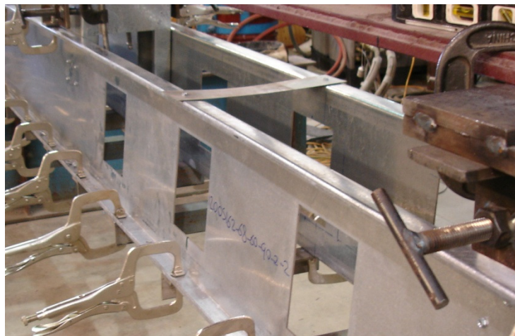
Figure 2.13 Cold-formed steel strap connecting two beams at mid-length
