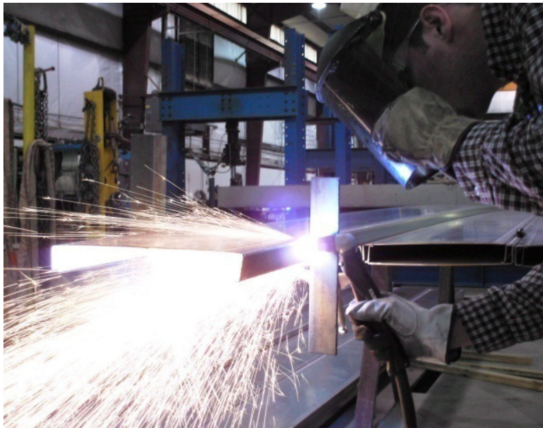
Figure 2.16. Rough cutting of the coupons using plasma cutter (Bowen 2009)
