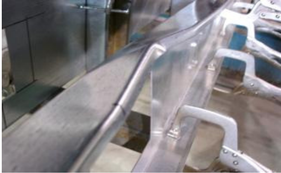
Figure 4.3. Distortional buckling failure
