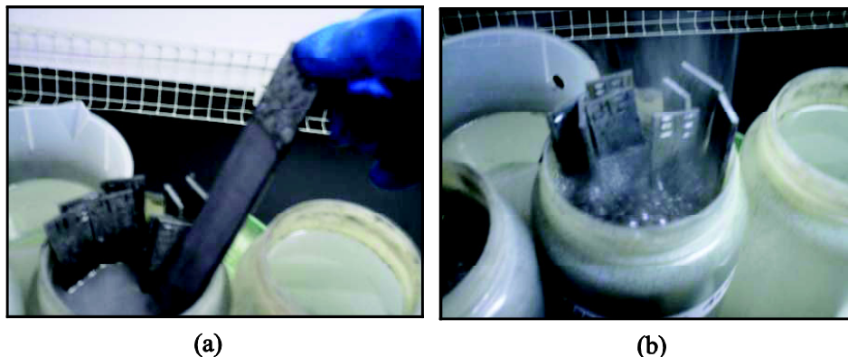
Figure 2.7. The zinc stripping process described in ASTM A90 – 07: (a) the reaction between the acid and the galvanic coating, (b) the coating has been removed exposing the base metal
