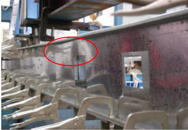
Figure 4.6. Unstiffened strip local buckling in 1000S162-54-95-1
