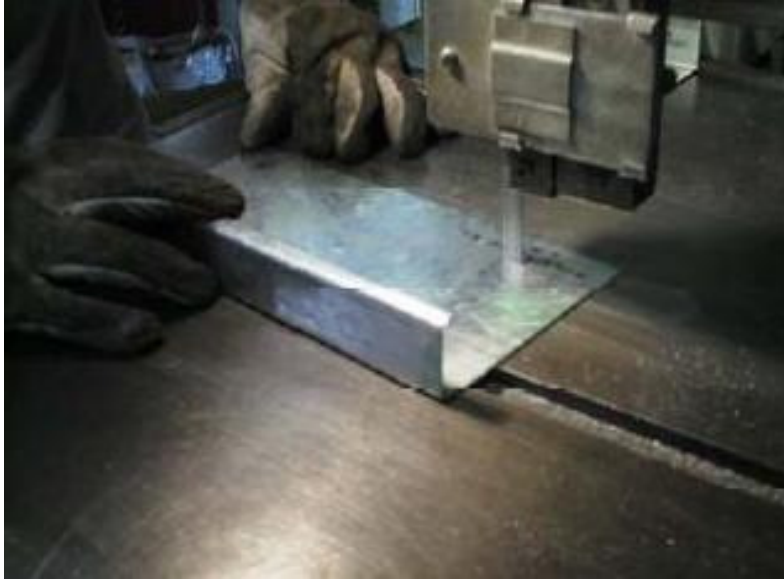
Figure 2.17. Rough cutting of coupons using band saw (Bowen 2009)
