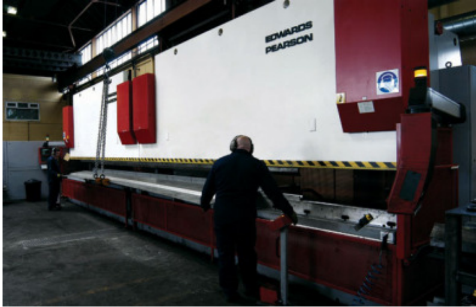
Figure 1.1. Press-braking of cold-formed steel sections (photo courtesy of Folsana)
