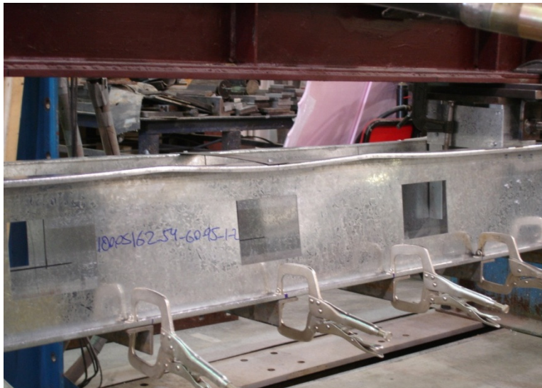
Figure 4.7. Distortional buckling in 1000S162-54-95-1
