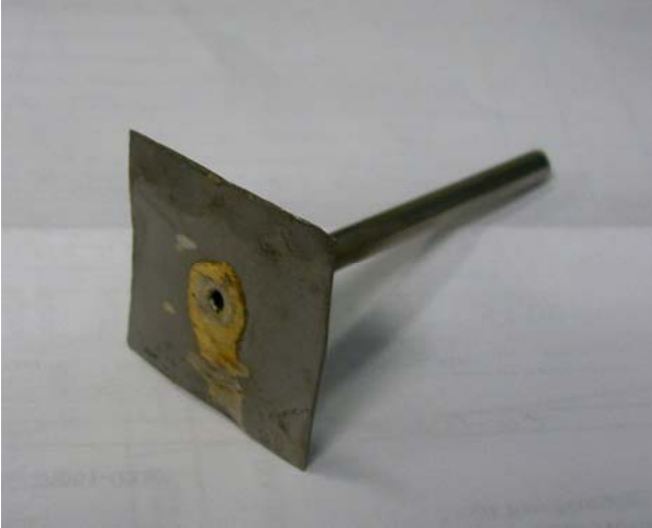
Figure 13 E-brite stainless steel Cu-Zn brazed to ¼” stainless steel tubing
