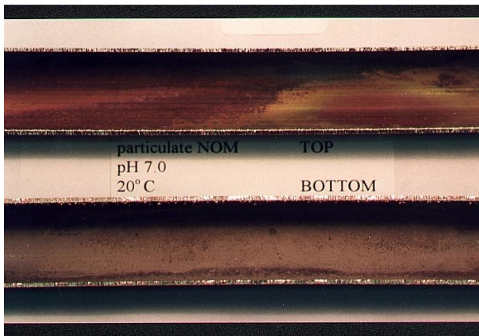
Figure 2-7: The top and bottom sections of pipes exposed to particulate NOM. The bottom section contained a dense layer of particulate matter that had settled from solution, while the top layer was multi-colored and coated with black particles.
