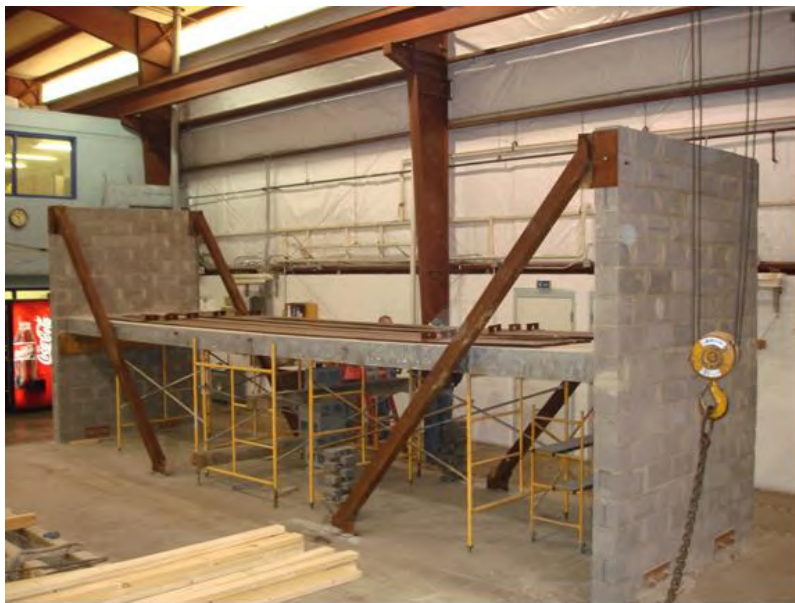
Figure 3.11 Static Tests, Distributed Load (Stage 3)
