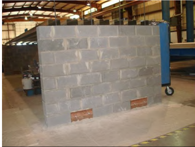
Figure 3.5 Construction of the CMU Walls
