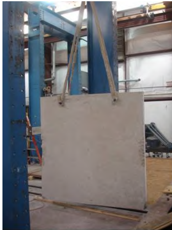
Figure 3.25 Vibration Tests in the Slab Section
