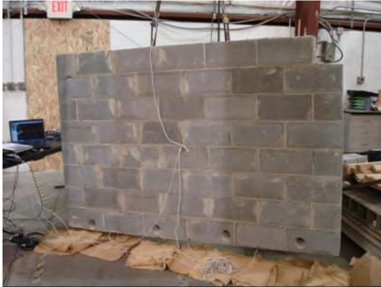
Figure 3.24 Vibration Tests in the CMU wall
