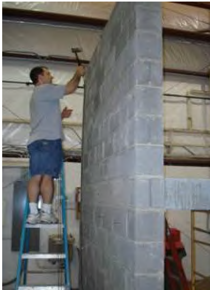
Figure 3.14 Strike in the Structure with the Impulse Hammer
