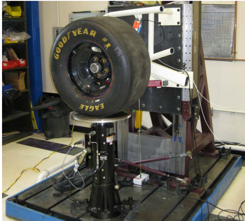
Figure 3.1: Quarter Car Test Rig
