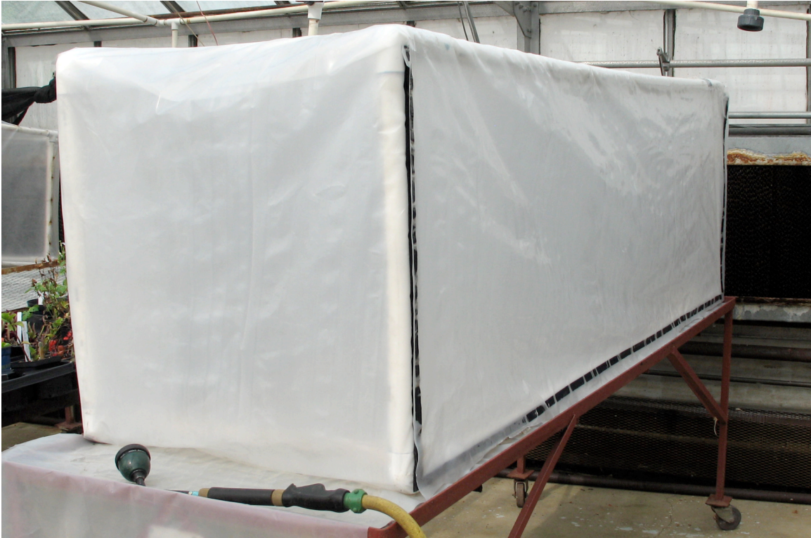
Figure 3.2 Chamber used for increasing temperature and humidity to encourage disease development. Chamber was composed of PVC pipe and plastic sheeting.
