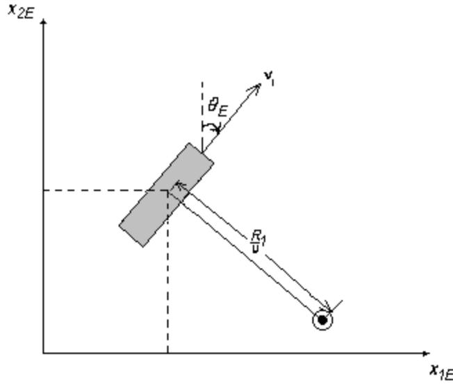
Figure 3.3: Global coordinate system and parameters for rolling disc model
