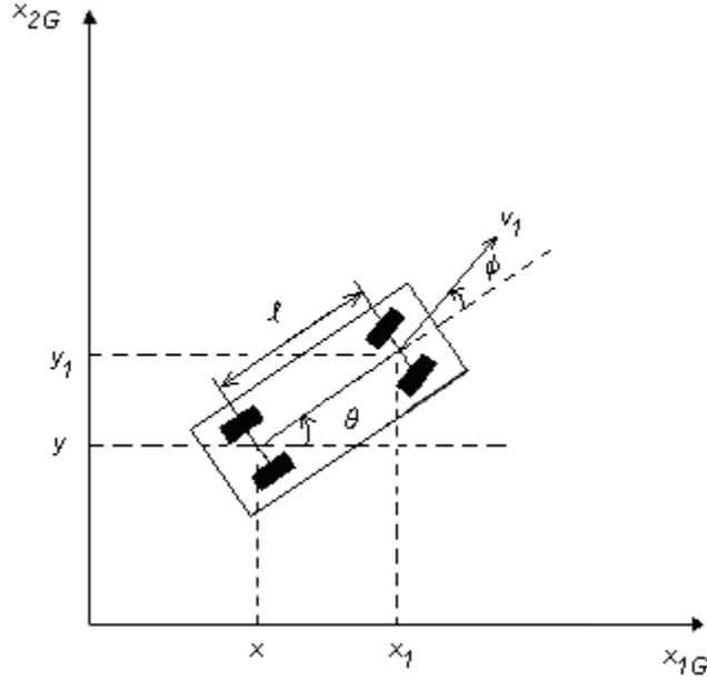
Figure 3.1: Global coordinate system for robotic vehicle [9]
