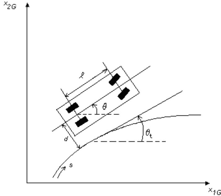
Figure 3.2: Path following coordinate system for robotic vehicle [9]
