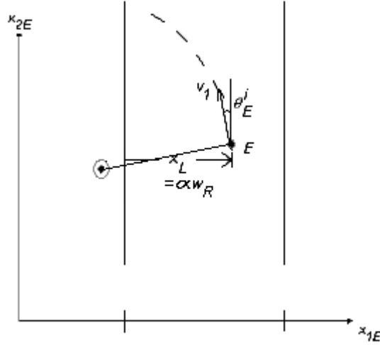
Figure 6.1: Real space tracking of vehicle; e.g.  $x_L$  distance to left edge
