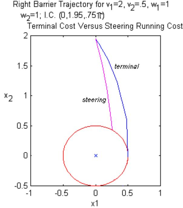
Figure 6.2: Comparison of terminal cost and steering cost for E on a straight path
