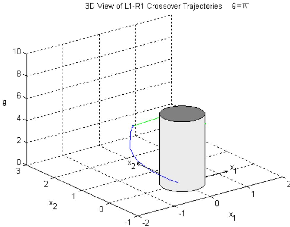
Figure 5.6: Left and right crossover trajectories; case of non-identical vehicles ( $v_1 = 1.5$ ,  $\omega_1 = 2$ ,  $v_2 = 1$ ,  $\omega_2 = 4$ )
