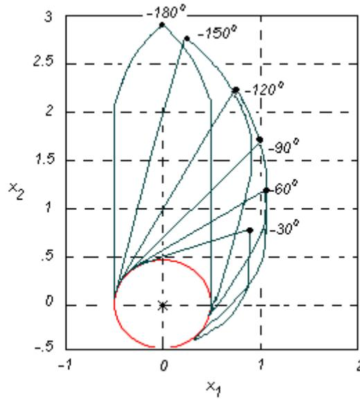
Figure 5.9: Left and right barriers for  $\theta_0 \in [0, -\pi]$ ; case of identical vehicles
