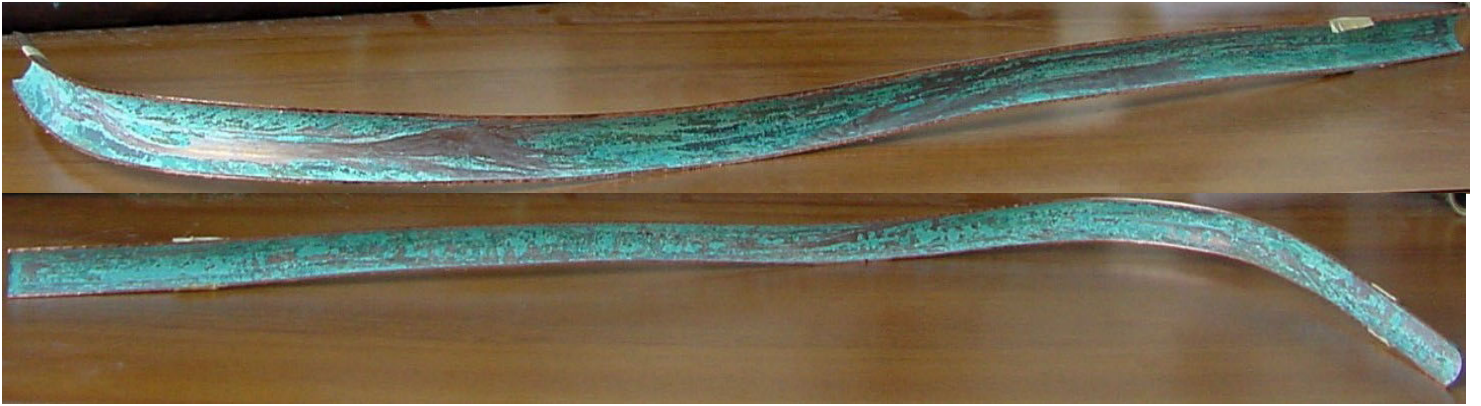
Figure 3-17. Free Chlorine Control System – Pipe Section.
