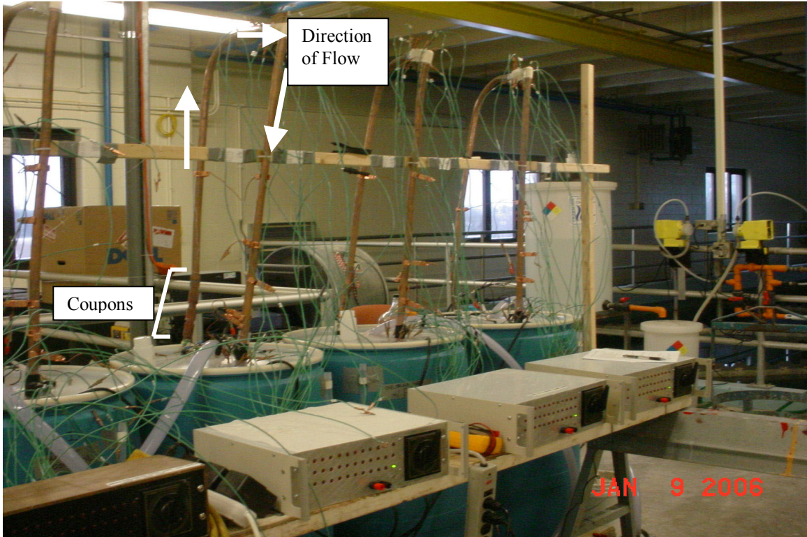
Figure 3-1. General pitting rig experimental setup with relay boxes.
