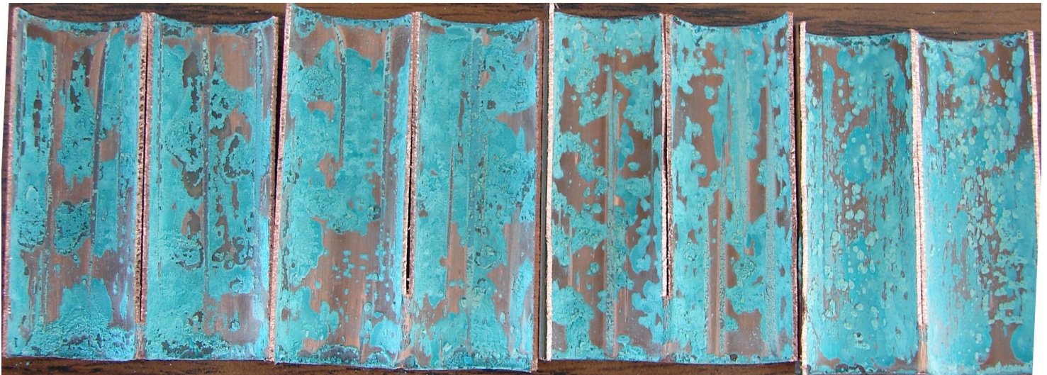
Figure 3-11. Free Chlorine Control System - Coupons. Coupons A – D shown left to right.
