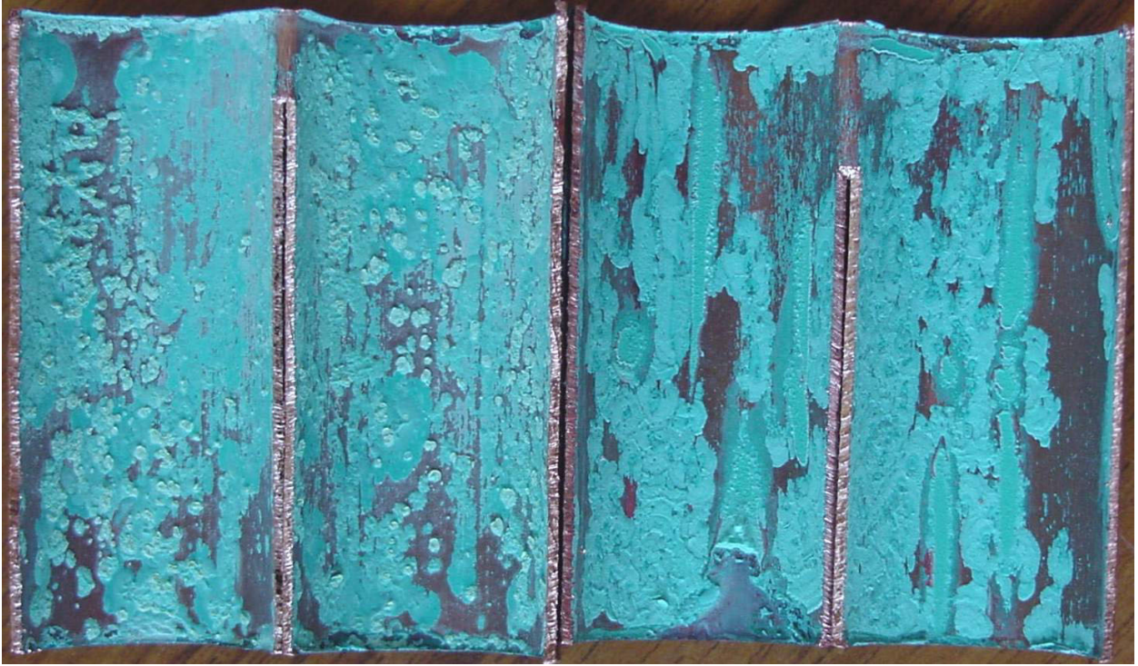
Figure 3-15. Free Chlorine Systems – Coupon D Comparison. Free chlorine control system (left) and free chlorine system with inhibitor (right).
