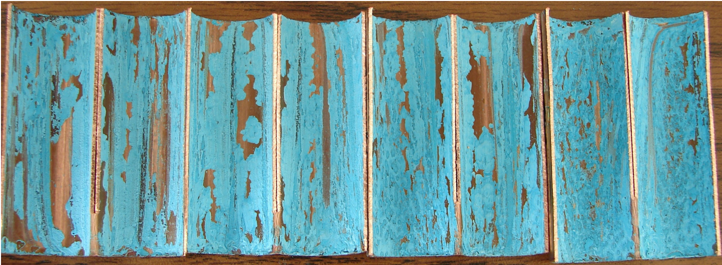
Figure 3-12. Chloramine System with Inhibitor - Coupons. Coupons A – D shown left to right.
