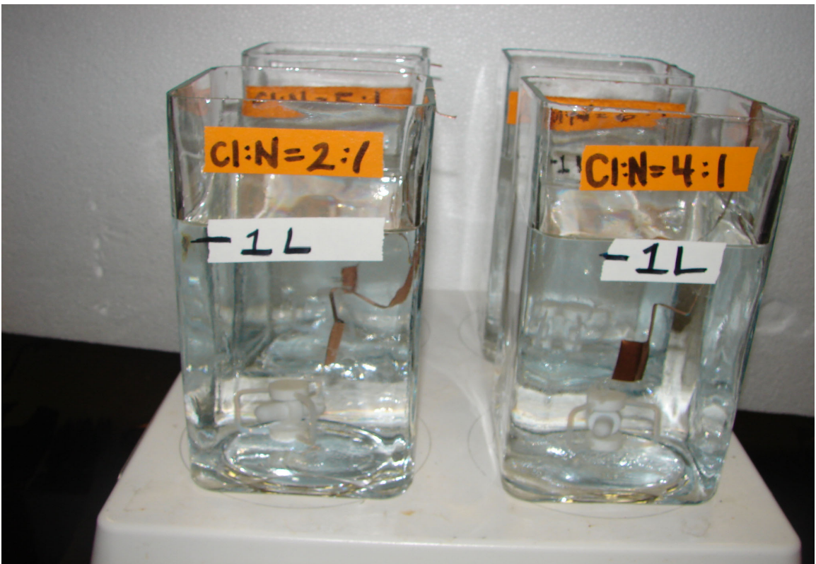
Figure 2-4. Jar tests with copper coupons installed.
