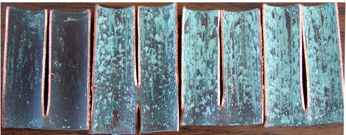
Figure 2-27. Orthophosphate-Polyphosphate Rig Coupons. Coupons A – D shown left to right.
