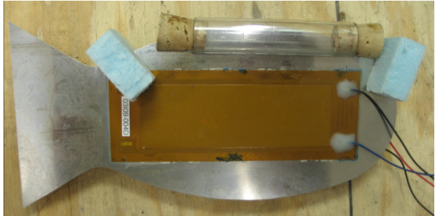
FIGURE 4.1 PROTOTYPE CARANGIFORM SWIMMER.
