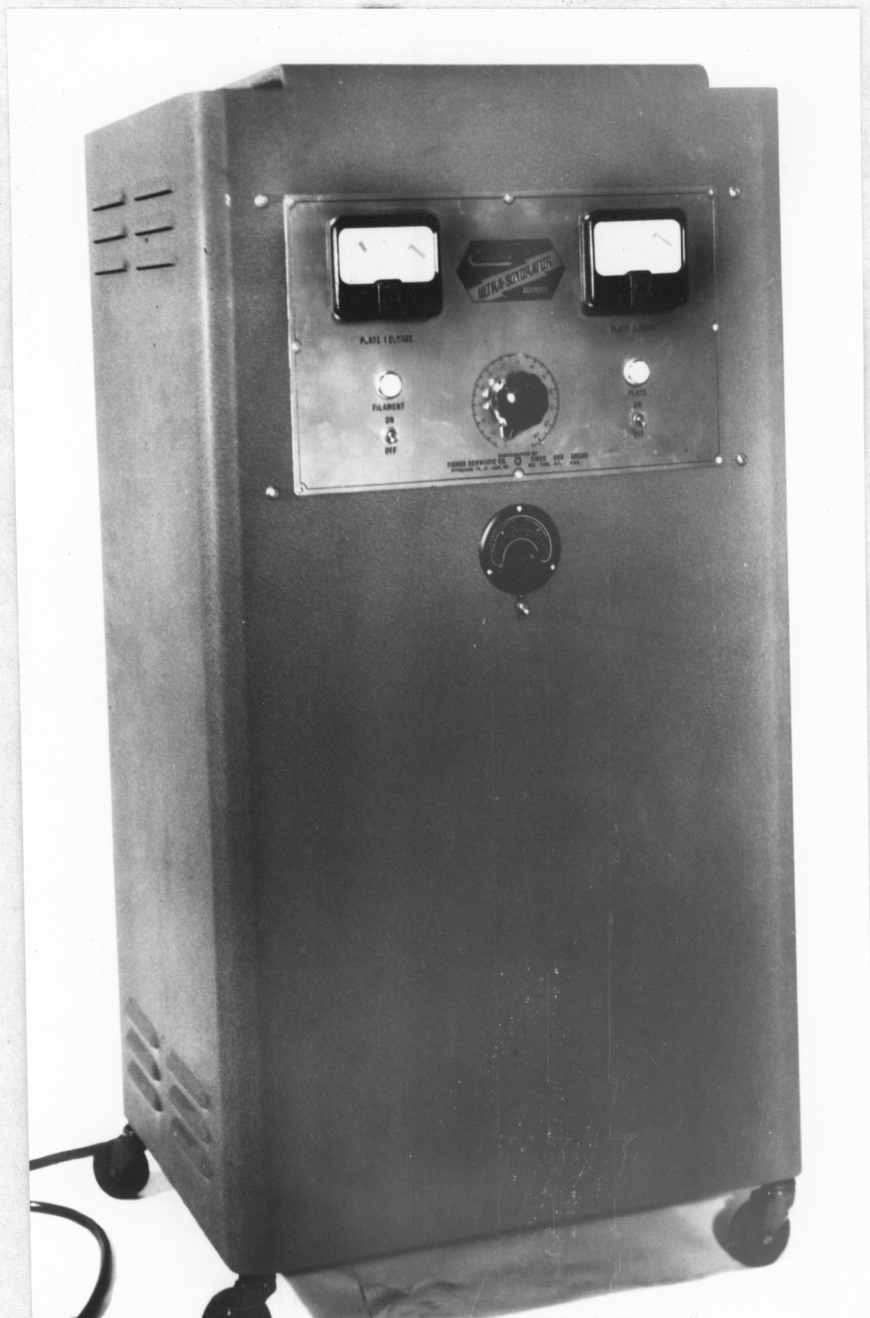
Figure 15. Front View of Ultra-Sonorator High Frequency Generator Showing Plate Voltmeter (left), Plate Ammeter (right), Switches, Powerstat, and Timer (lower center).
