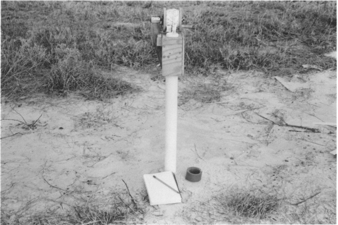
Fig. 10 Meter in place on well for taking a level reading.
