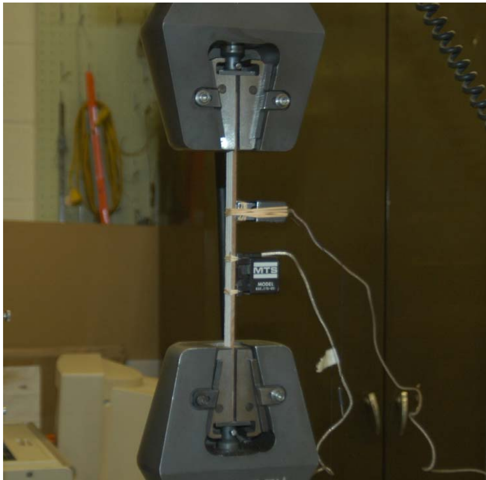
Figure 11: Test Setup for Measurement of v_{xz}
