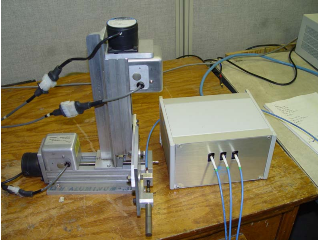
Figure 4.6: Ocean Optics S2000 Spectrometers and Velmex Unislide Traverse System Fitted with the Spectrometer Scope
