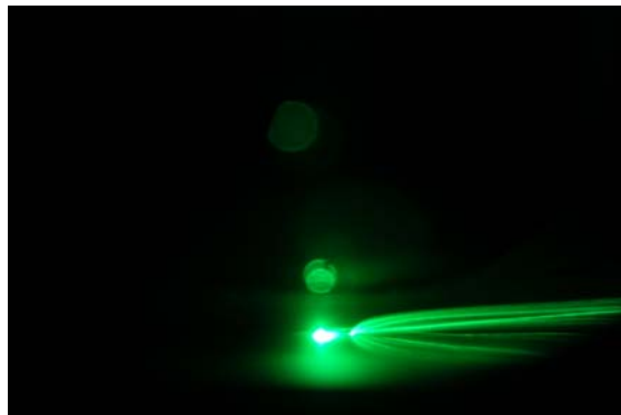
Figure 5.17: A Filtered Photograph Displaying Electrode Erosion in the Supersonic Environment with a Shutter Speed of 1/500 and a Band Pass Filter Centered at 515.1 nm
