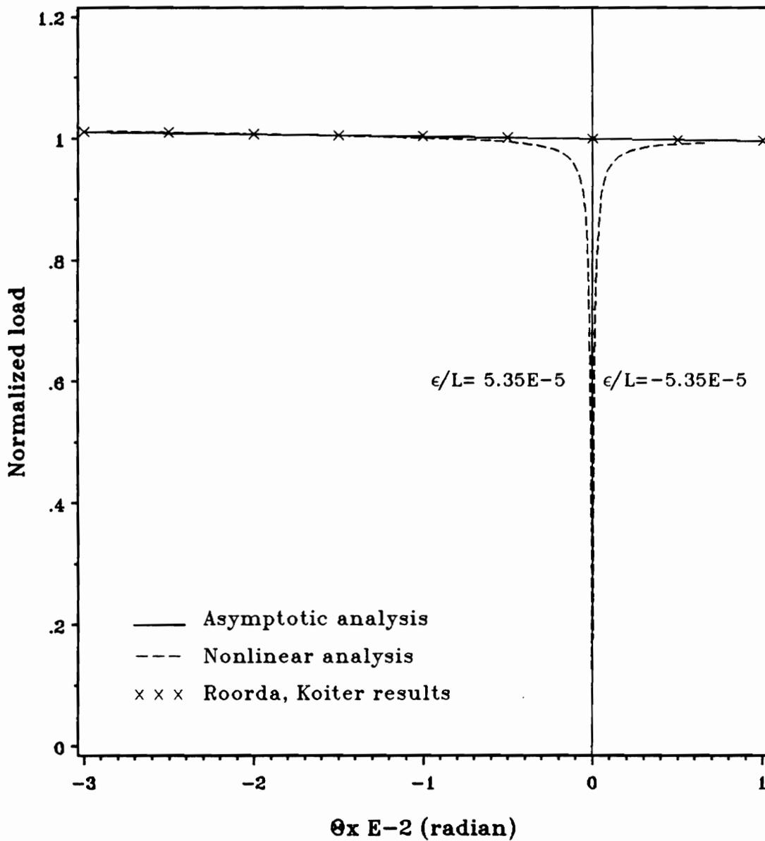
Figure 13. Load-displacement behavior for knee frame
