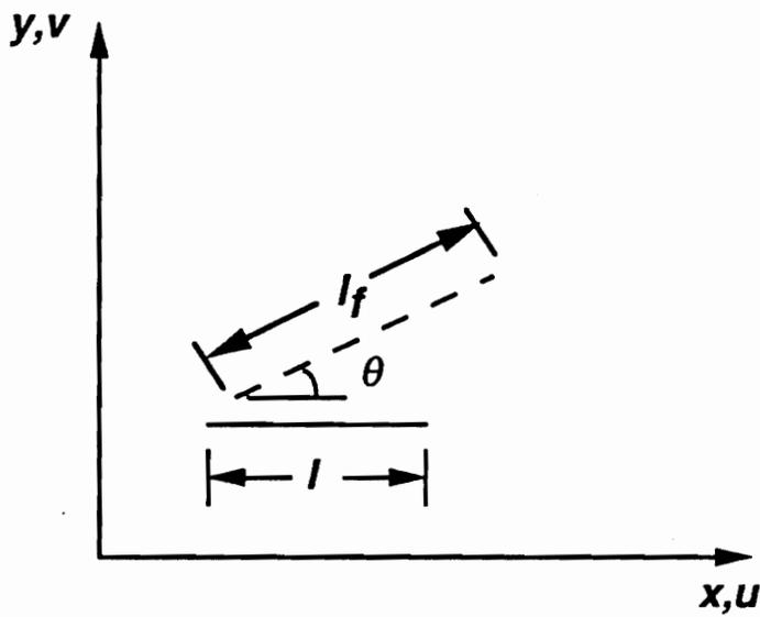
Figure 7. Truss element in X-Y plane
