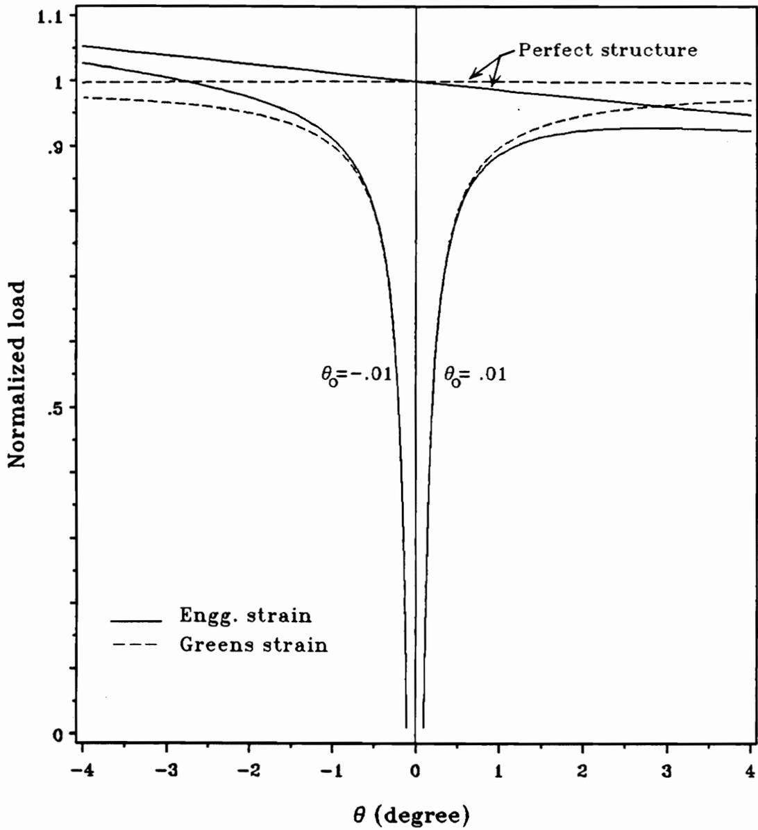
Figure 3. Load-displacement behavior for one degree of freedom model
