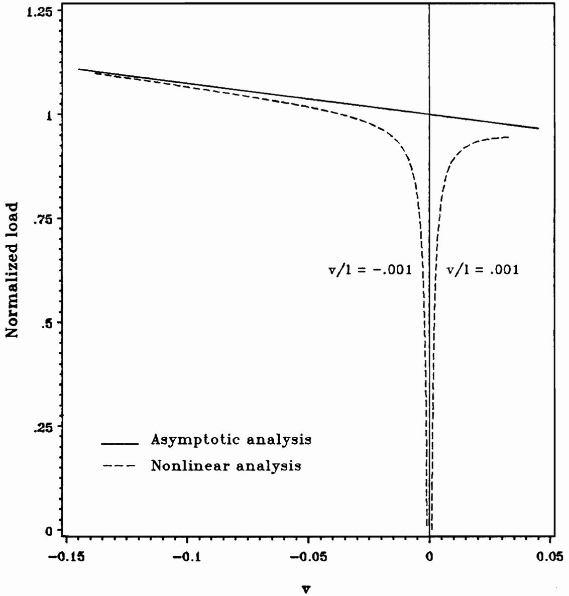
Figure 9. Load-displacement behavior for spring bar structure
