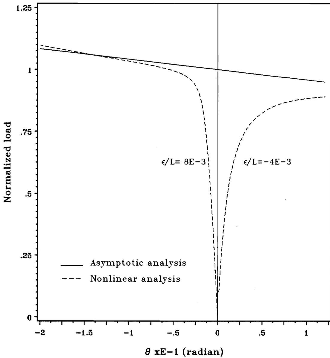
Figure 11. Load-displacement behavior for knee truss
