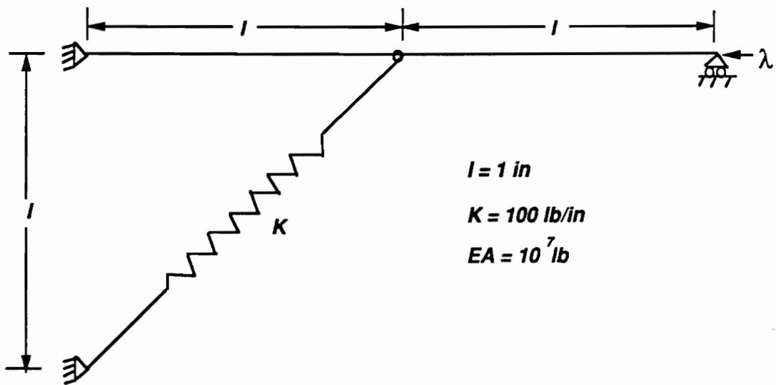
Figure 8. Spring bar structure
