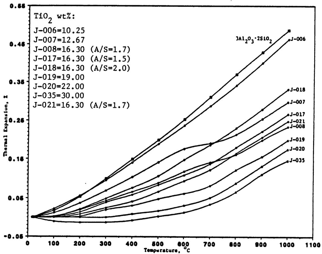
Figure 6. Thermal expansion of mullite-based bodies containing  $Al_2TiO_5$ .
