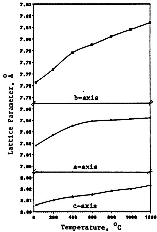
Figure 9. Axial expansion for  $\text{Ga}_2\text{O}_3$ -modified mullite solid solution.
