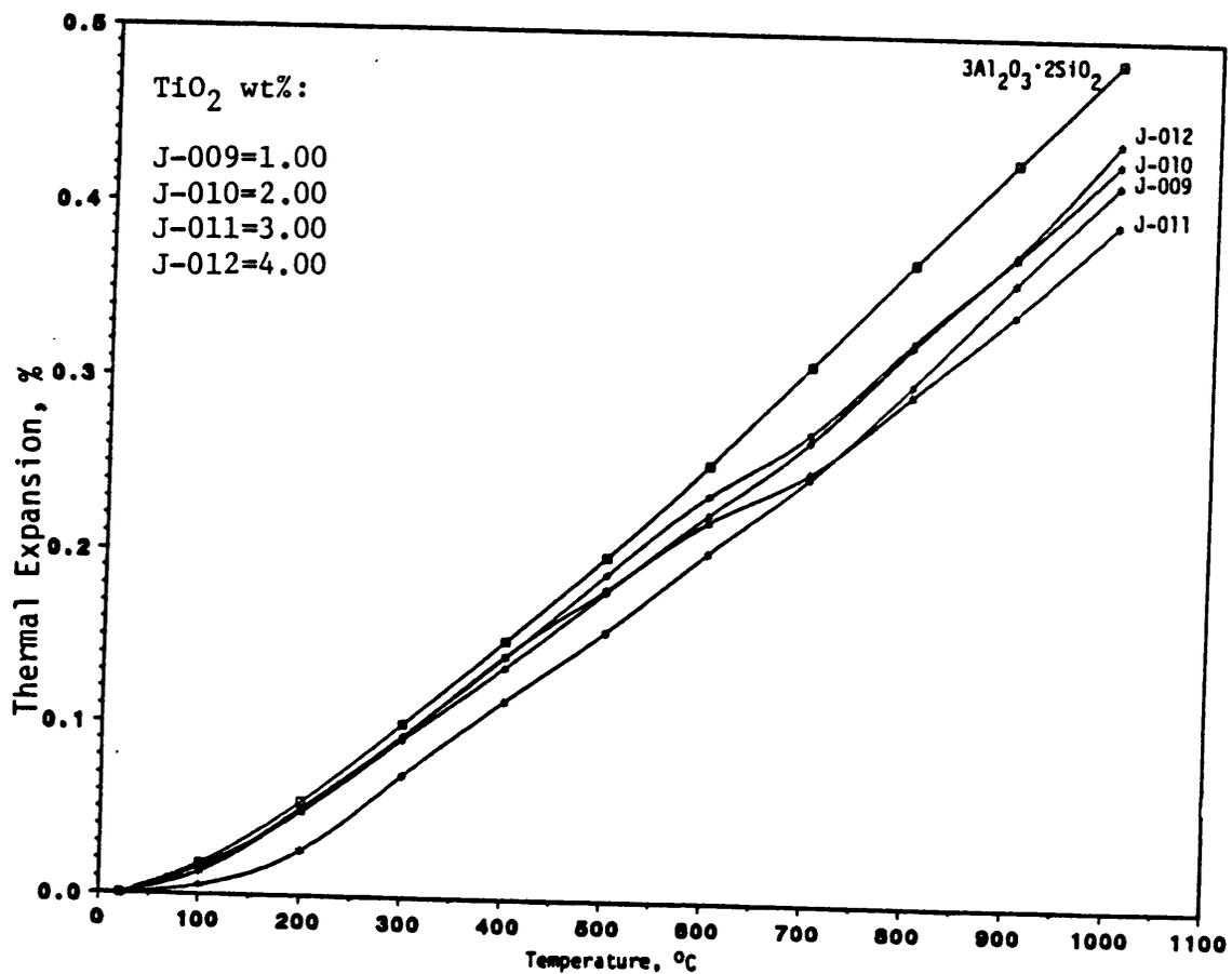
Figure 5. Thermal expansion of TiO<sub>2</sub>-modified mullite solid solutions.
