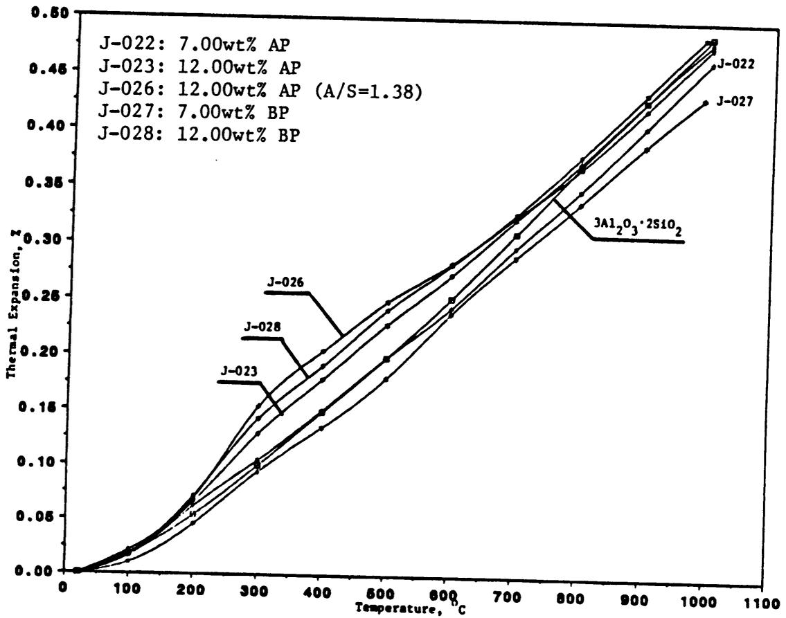
Figure 8. Thermal expansion of  $AlPO_4$ - $BPO_4$ -mullite-based system.
