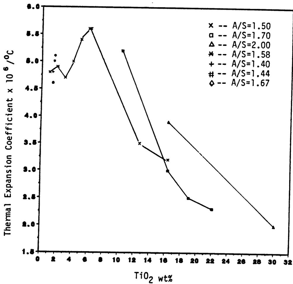
Figure 11. CTE in the TiO<sub>2</sub>-mullite-based system with varying Al<sub>2</sub>O<sub>3</sub>/SiO<sub>2</sub> molar ratio.
