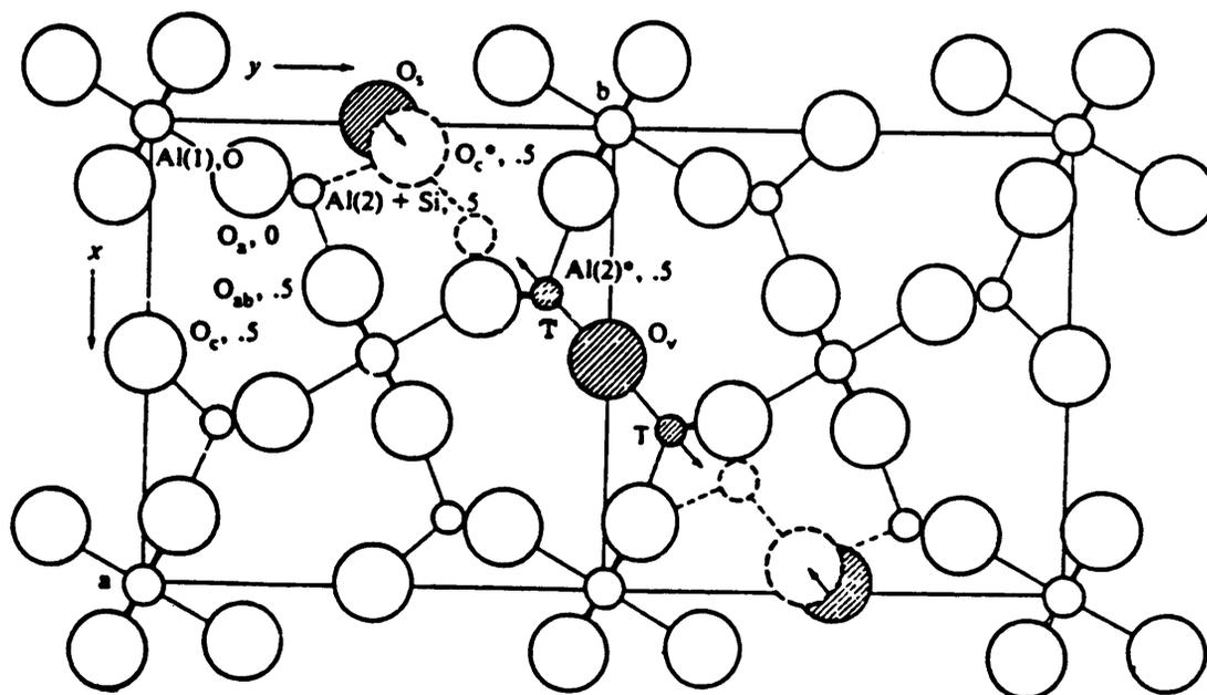
Figure 1. Project on (001) of the mullite structure; two unit cells show the effect of removing one  $O_c$  atom.  $O_v$  = oxygen removed,  $T$  = untenable tetrahedral site,  $O_s$  = oxygen shifted.<sup>45</sup>
