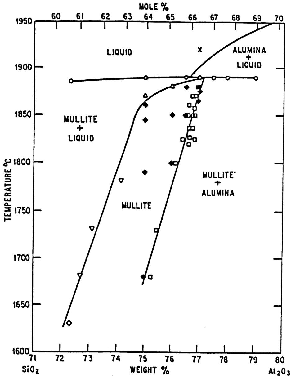
Figure 2. The Al<sub>2</sub>O<sub>3</sub>-SiO<sub>2</sub> phase diagram in the mullite(ss) region at T ≥ 1600°C showing solid solution boundaries to be temperature-dependent.<sup>4</sup>
