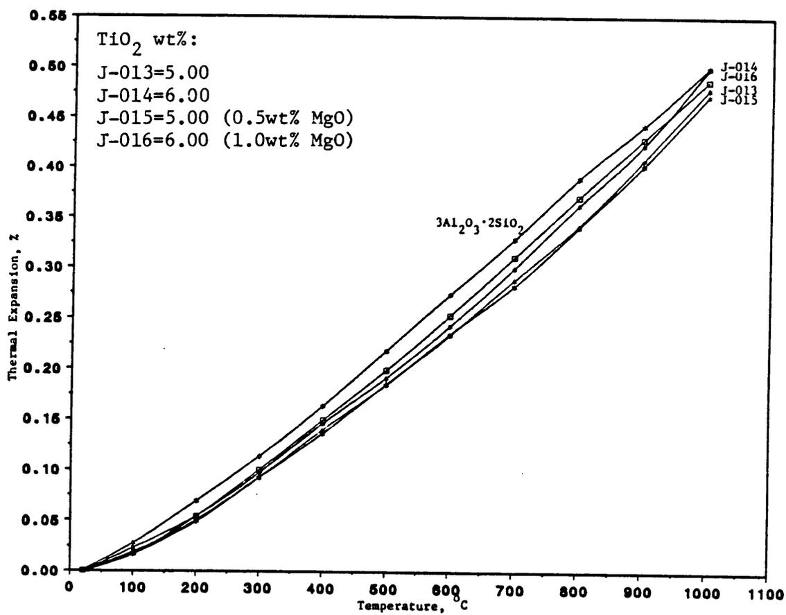
Figure 7. Thermal expansion of TiO<sub>2</sub> modified mullite solid solutions with/without MgO.
