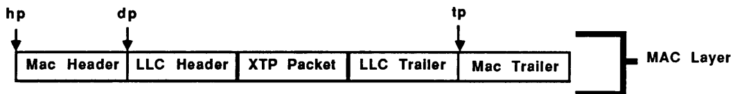
Figure 23. Receive pbuf Pointer Initialization at the Mac Layer
