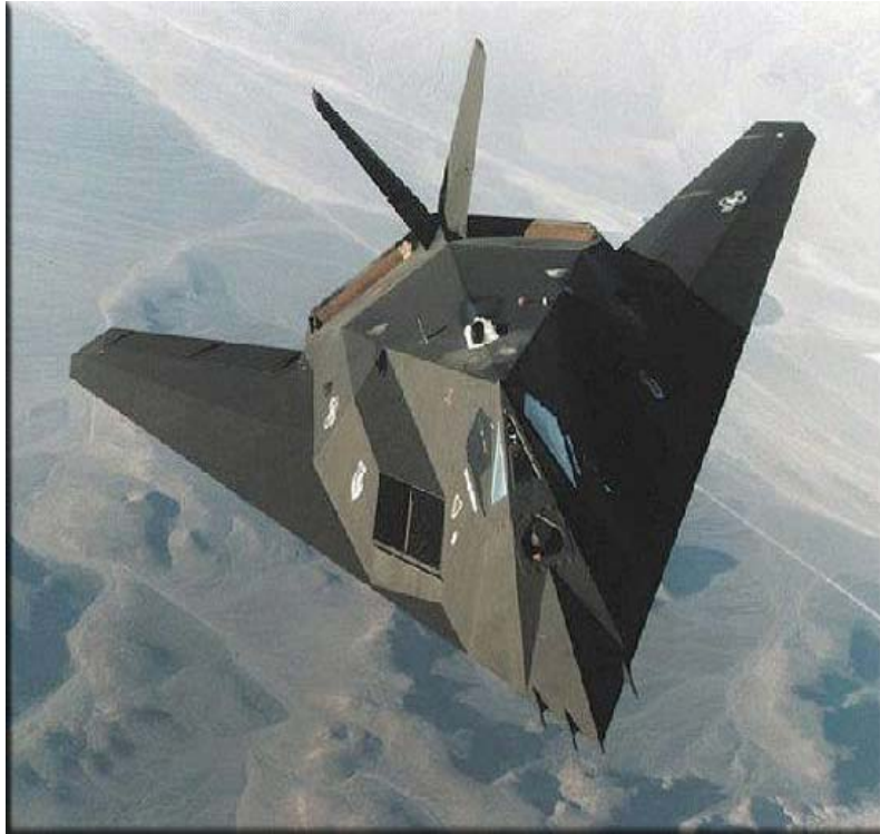
Figure 1-2: F117 Nighthawk has an 'S' shaped or stealth inlet, increasing the potential for the inlet flow to its engines to be non-uniform [ www.aladdinssoft.com ].
