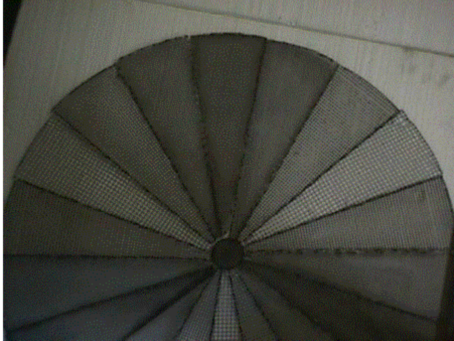
Figure 5-6: Example of a 3 per rev distortion screen [Morrow, 1993].
