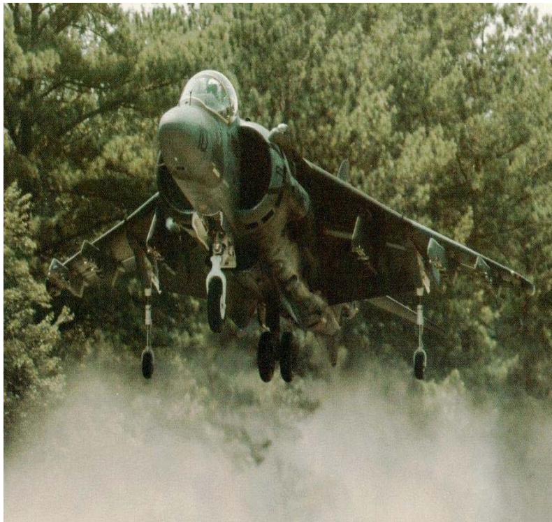
Figure 1-3: The AV-8B Harrier. The ingestion and subsequent mixing of the hot exhaust gases with the cooler atmospheric air could cause the inlet pressure profile to the aircraft's engine to be non-uniform [ www.globalsecurity.org ].
