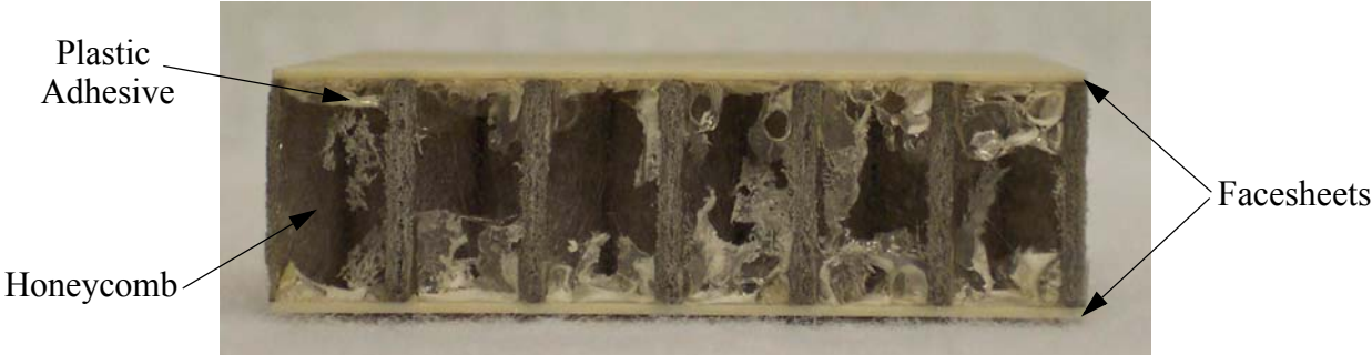
Figure 4.14: Scotch-Grip™ plastic adhesive sandwich specimen
