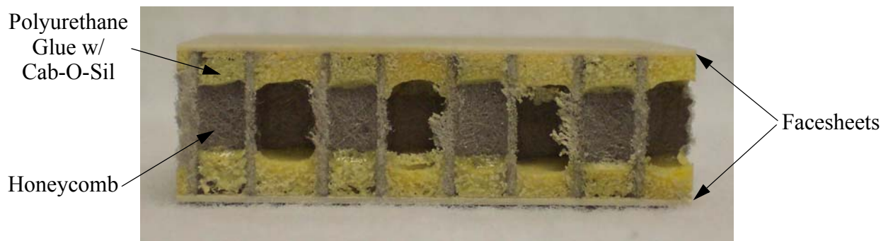
Figure 4.12: Polyurethane glue with Cab-O-Sil sandwich specimen
