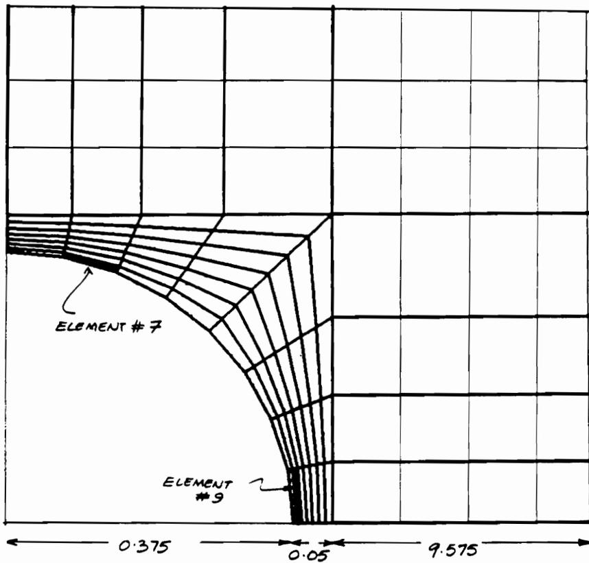
Figure 6. Mesh Used for EBE PCG and EAL Stress Comparison
