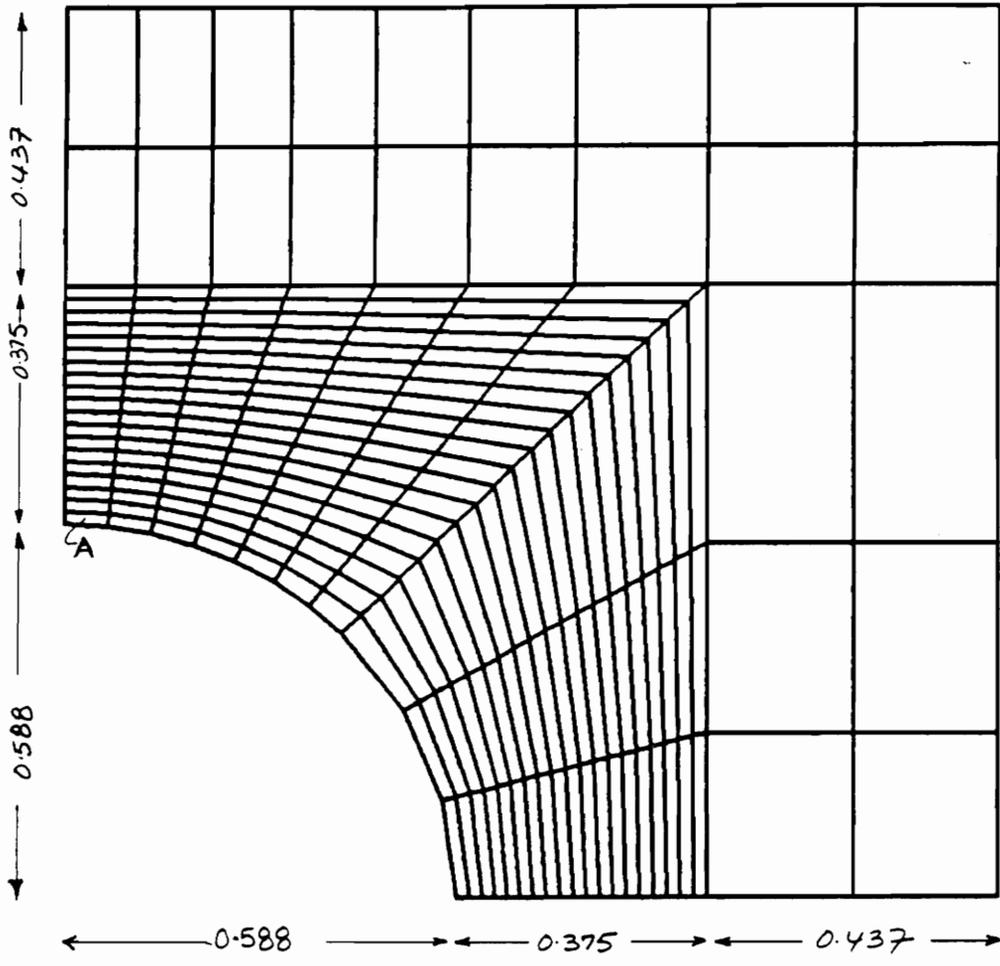
Figure 5. Mesh Discretization - Initial Design
