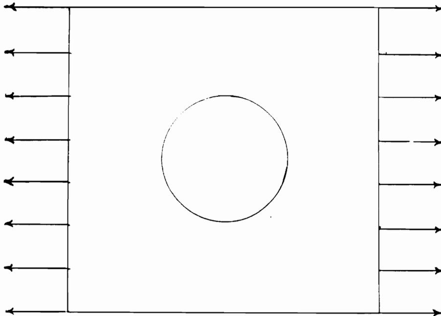
Figure 4. Plate with a Central Hole Subjected to Uniform Loading
