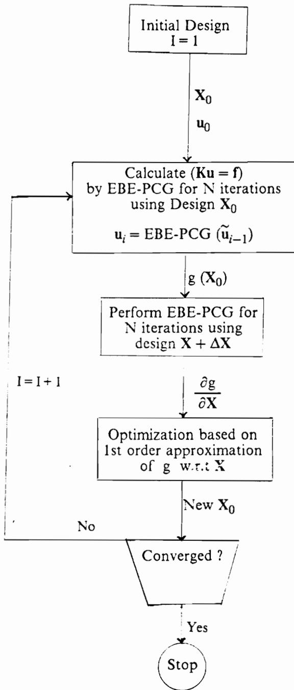
Figure 3. Flow Chart for Integrated Analysis and Design
