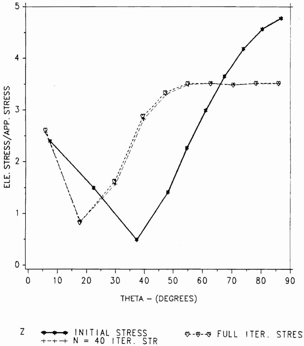
Figure 14. Stress Concentration in Elements Around Hole Boundary (Inexact Forces)
