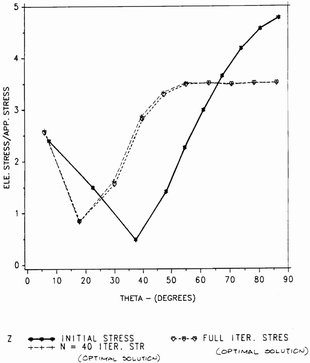
Figure 11. Stress Concentration in Elements around Hole Boundary
