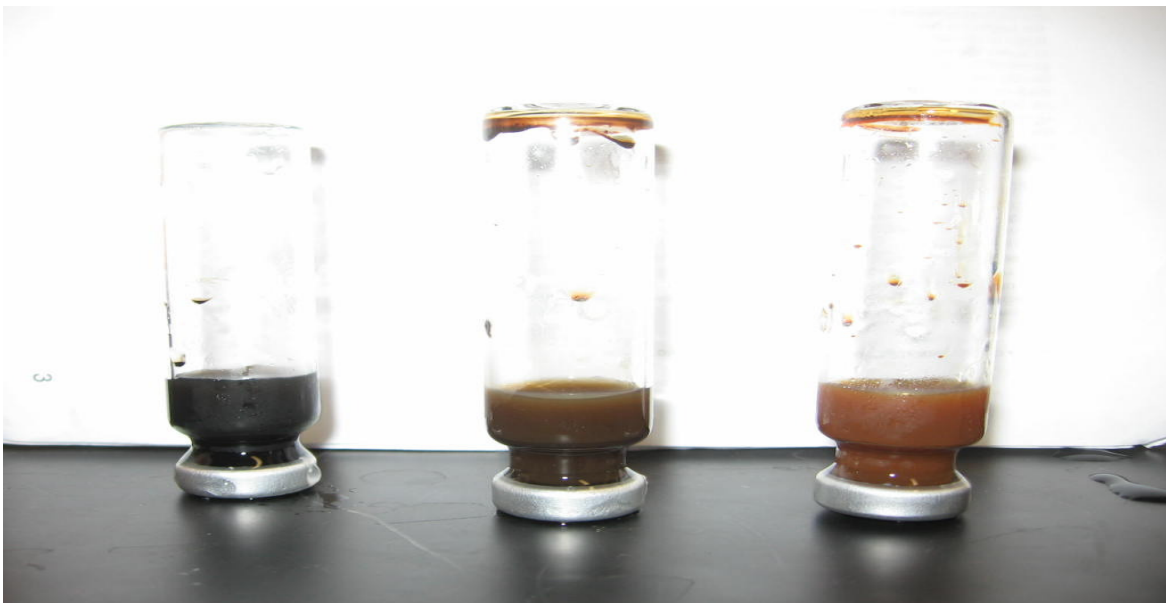
Figure 3-2. Magnetite oxidation samples. In order from left to right, magnetite at t = 0 , t = 3 hours of oxidation, and t = 10 hours of oxidation. Photograph by John Templeton.
