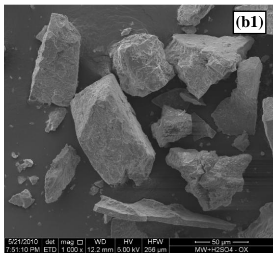
Figure 25. Scanning electron micrographs of solids precipitated from (a1) anaerobically digested manure (centrifuged); (a2) anaerobically digested manure (non-centrifuged); (a3) anaerobically digested manure pretreated with oxalic acid (centrifuged); (b1) raw manure (centrifuged); (b2) raw manure (non-centrifuged)
