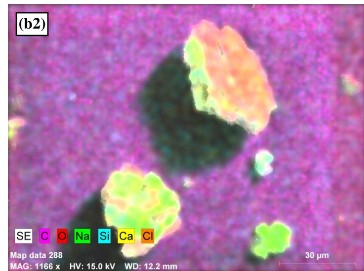
Figure 15. Energy dispersive X-ray mapping analysis of precipitated solids from different EBPR mediums: (a1) C - AML; (a2) NC - AML; (b1) C - Feed; (b2) NC - Feed.
