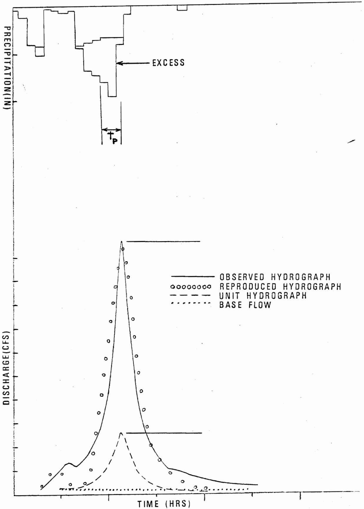
FIG. 1: DERIVATION OF A TYPICAL UNIT HYDROGRAPH (34)
