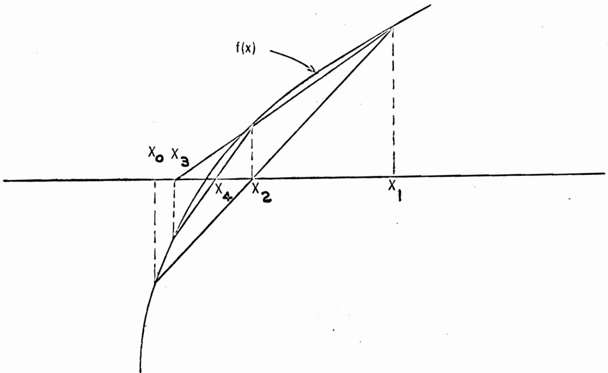
FIG. 9: GRAPHICAL REPRESENTATION OF THE METHOD OF SECANTS
