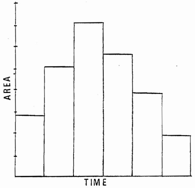
FIG. 2: DERIVATION OF THE TIME-AREA CURVE (28)
