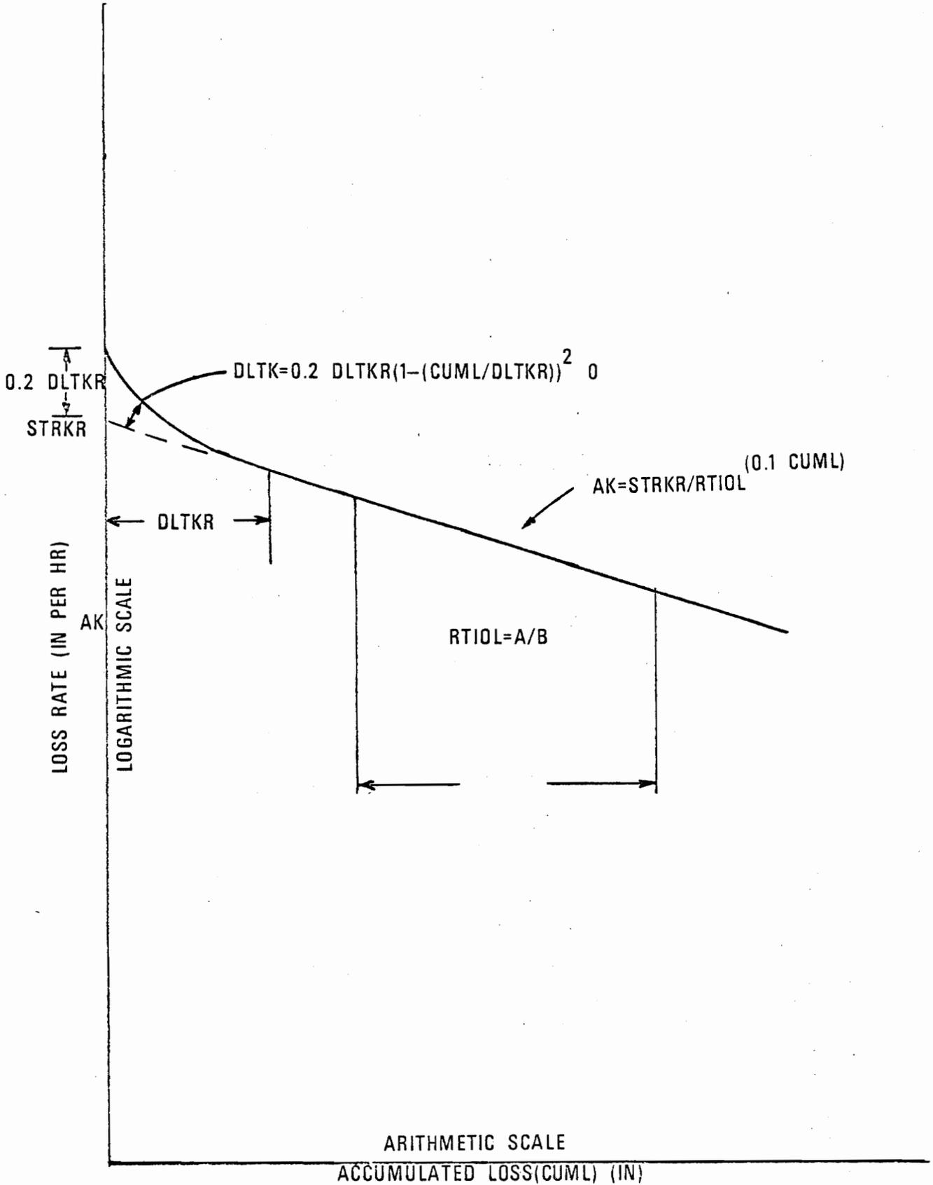
FIG. 7: GENERAL LOSS RATE FUNCTION ON SNOW-FREE GROUND(32)
