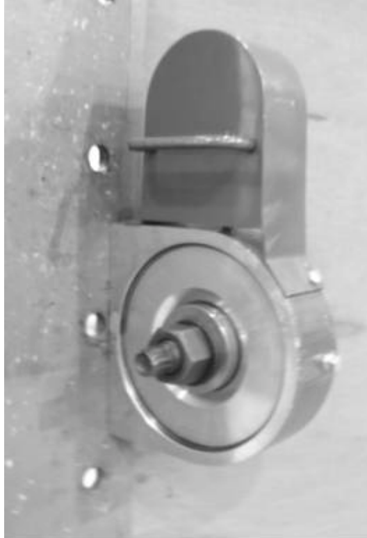
Figure F.1: Rear View of Typical Skidmore Setup
