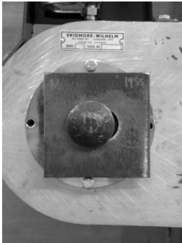
Figure F.4: Setup for 1" Bolt, A490 Strength, Off-Centered Test
