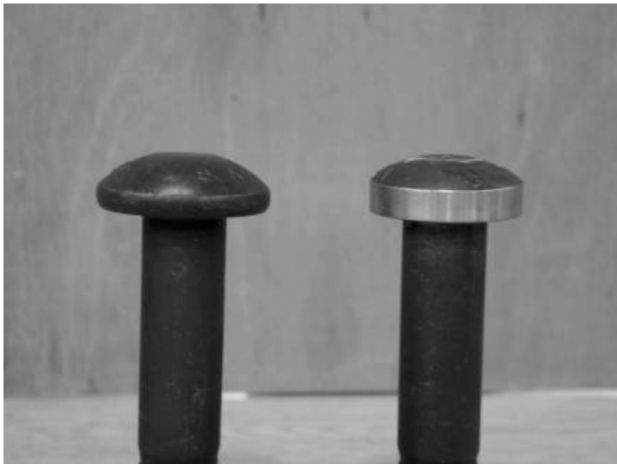
Figure F.2: Manufacturer's Standard and F1852 Minimum Bolt Heads
