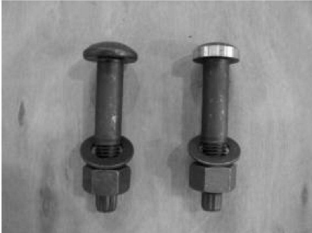
Figure 3.1: Photo of Manufacturer's Standard and Machined F1852 Minimum Diameter 1-1/8" Bolts
