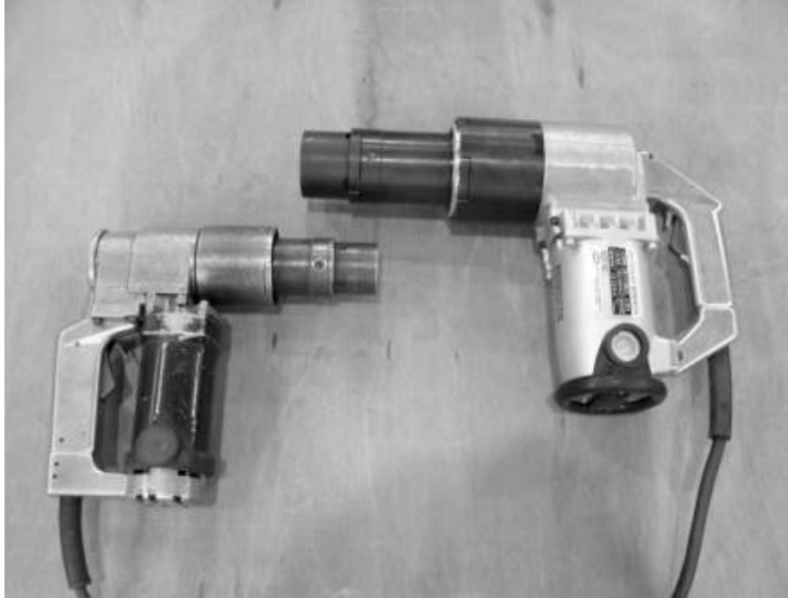
Figure F.3: Torque Wrenches Used for Tightening
