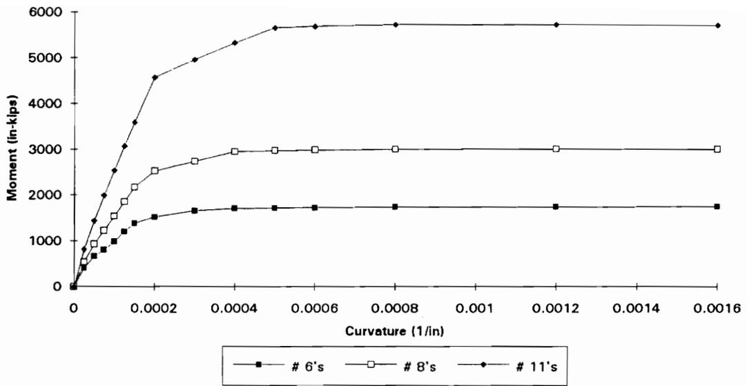
Figure 3.12 Moment-curvature for Beam-Column without Axial Load
