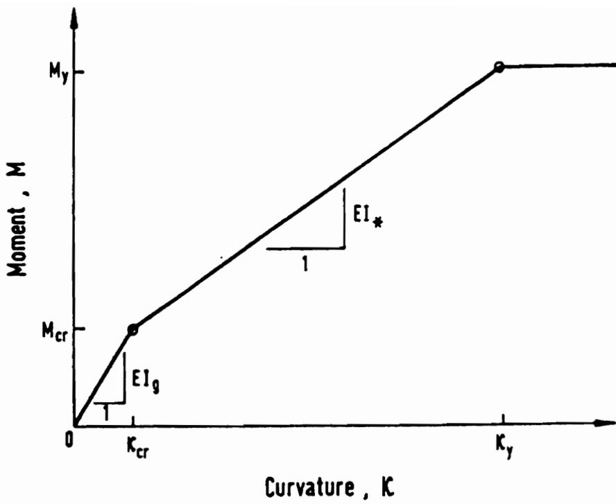
Figure 1.1. Trilinear moment-curvature model given by Alwis (1990)
