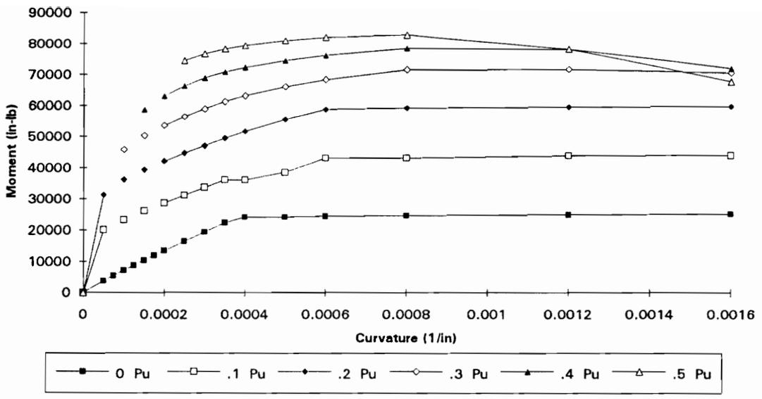
Figure 3.15 Moment-curvature for Beam-5 Section 1 with varying Pu
