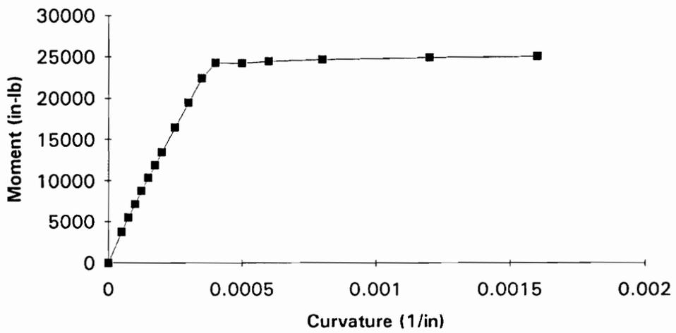
Figure 3.9 Moment-curvature curve for beam 5 (El-Metwally and Chen curves without tension)
