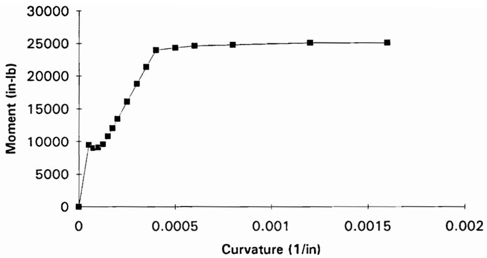
Figure 3.8 Moment-curvature curve for beam 5 (El-Metwally and Chen curves with tension)
