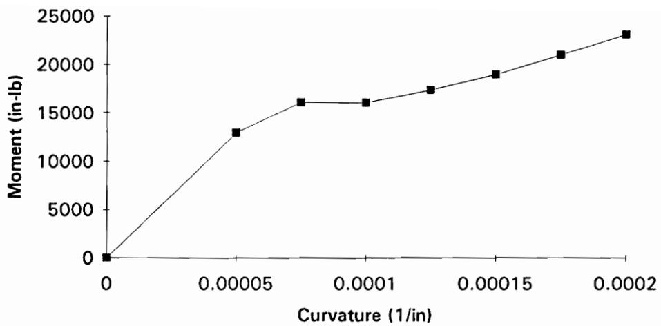
Figure 3.5 Moment-curvature curve for beam C1 with realistic tension curve
