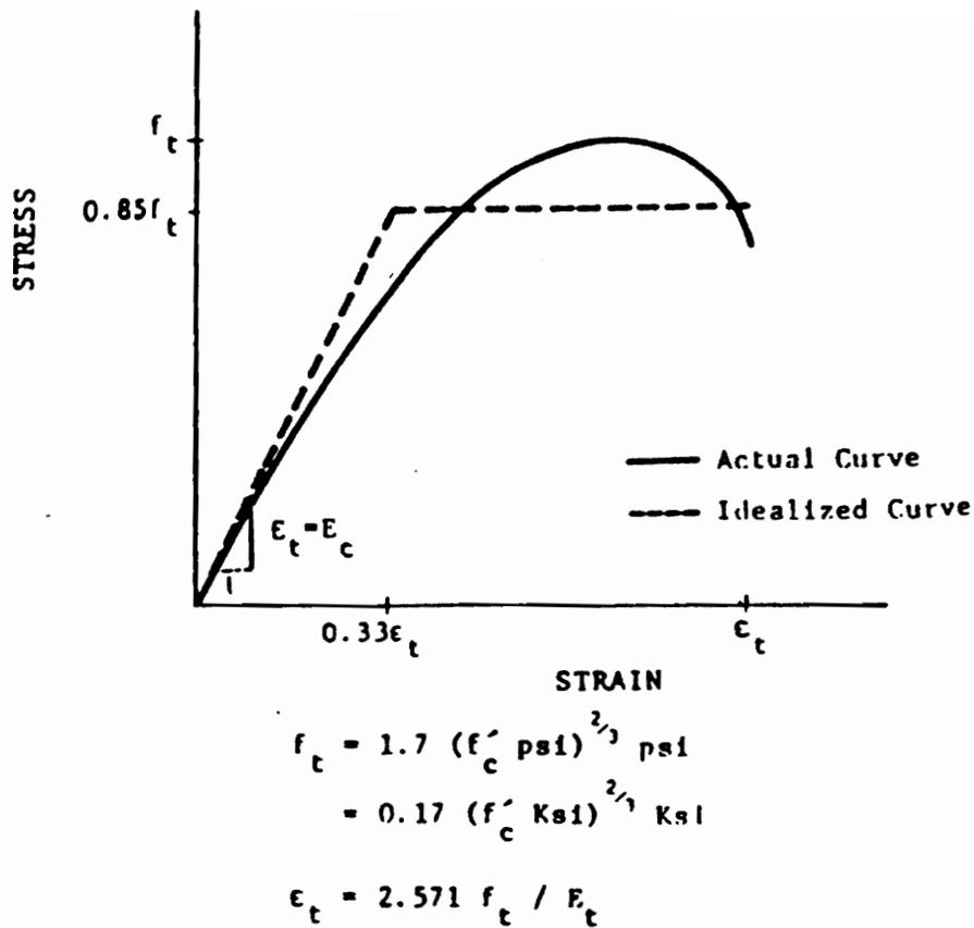
Figure 1.4. Stress-Strain Curve for Concrete in Tension adopted by El-Metwally and Chen
