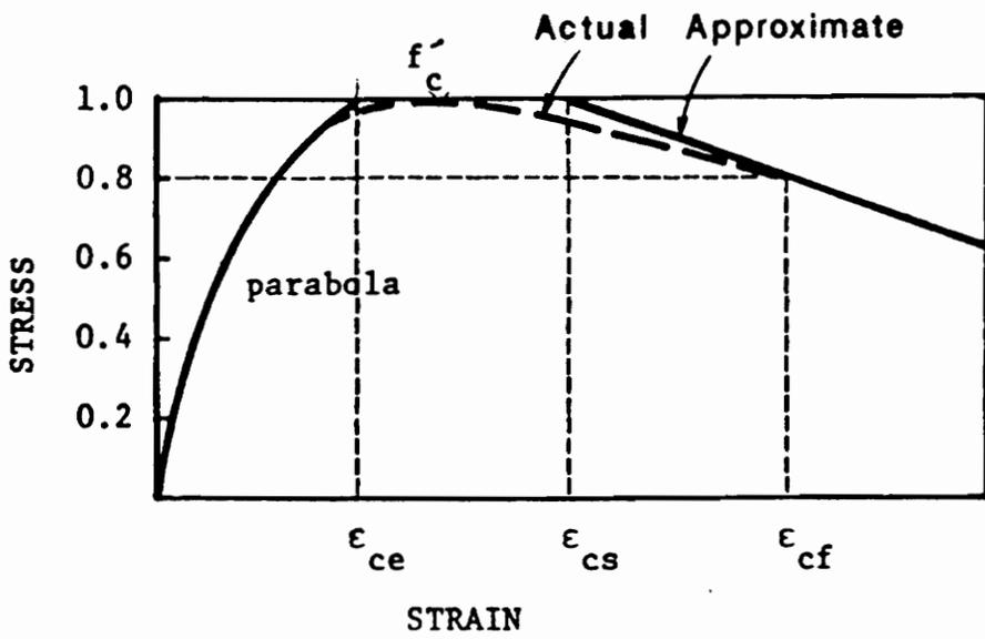
Figure 1.3. Stress-Strain Curve for Concrete in Compression adopted by El-Metwally and Chen
