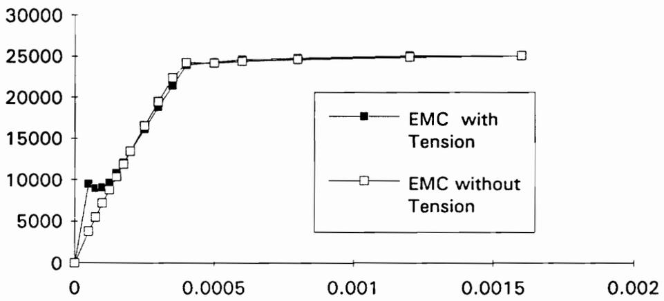
Figure 3.10 Moment-curvature curve for beam 5 with and without tension
