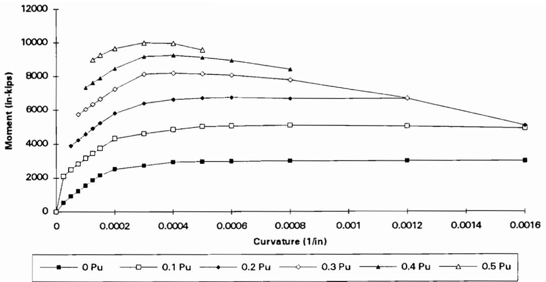
Figure 3.14 Moment-curvature for Beam-Column 8 #8's with varying Pu
