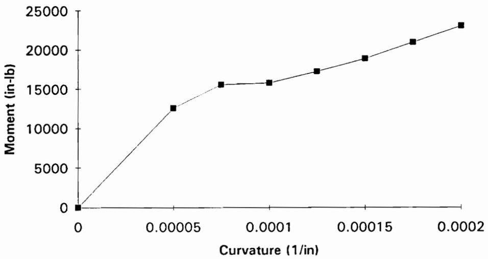
Figure 3.4 Moment-curvature curve for beam C1 with idealized tension curve
