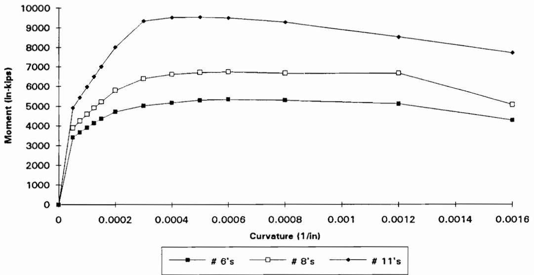
Figure 3.13 Moment-curvature for Beam-Column with 0.2 Pu
