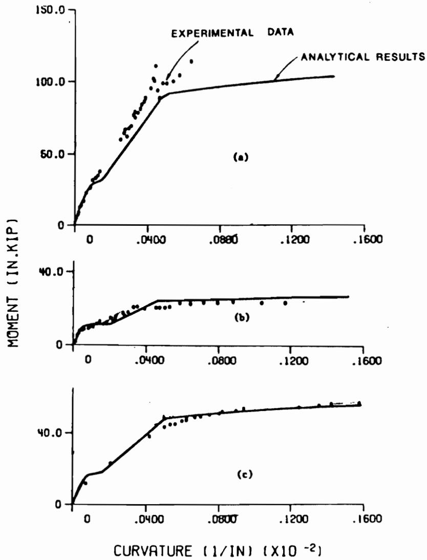
Figure 1.2. Analytic Moment Curvature relationship versus Experimental data.
