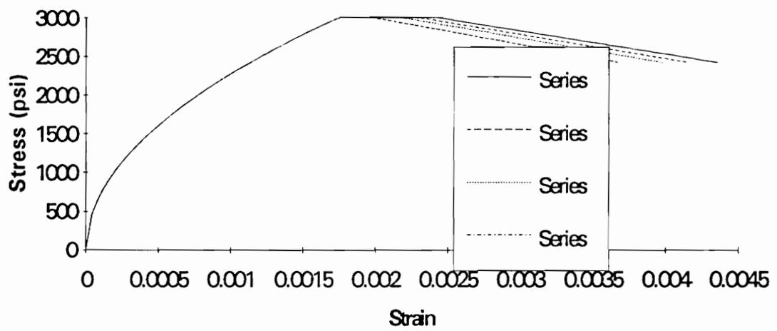
Figure 3.3 Stress-Strain curves for varying spacing of transverse steel
