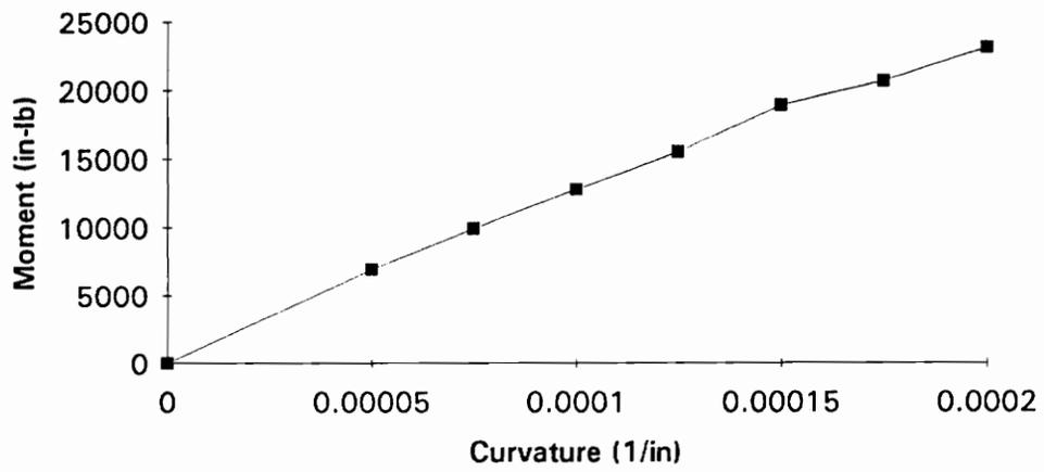
Figure 3.6 Moment-curvature curve for beam C1 with no tensile curve
