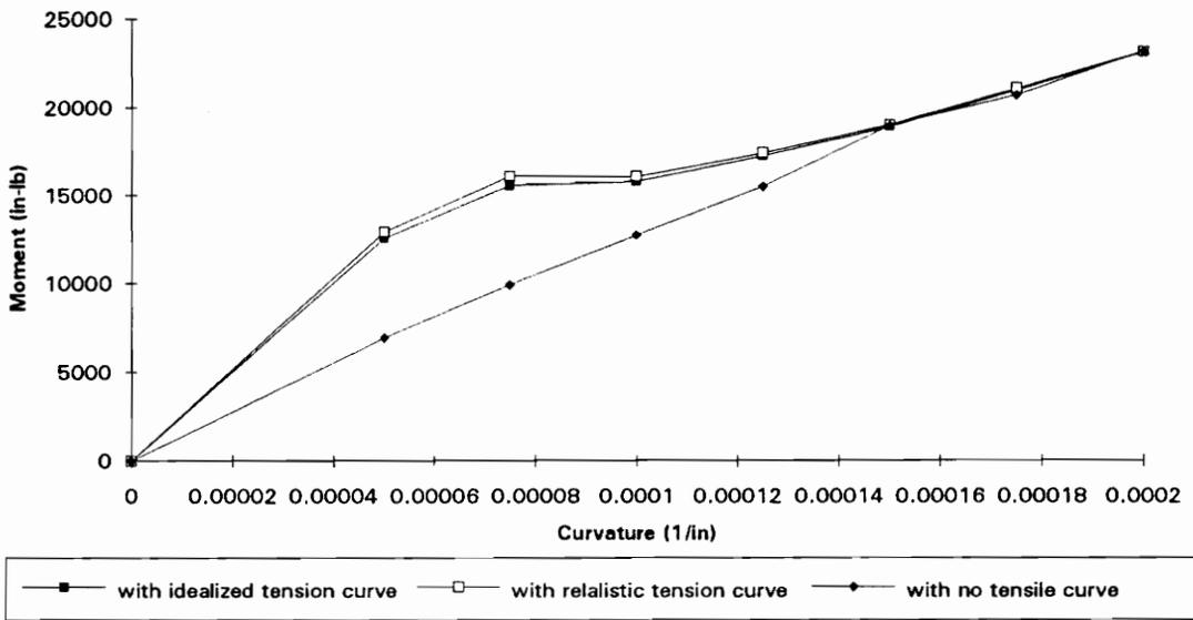
Figure 3.7 Moment-curvature curve for beam C1 with all three curves
