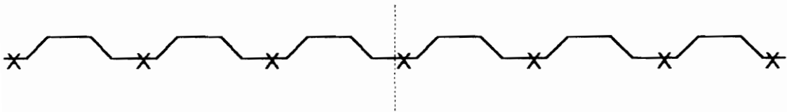
Figure A.121 SDI-2/20-PX2-9 Concrete Strain Gage and Arc Spot Weld Locations
