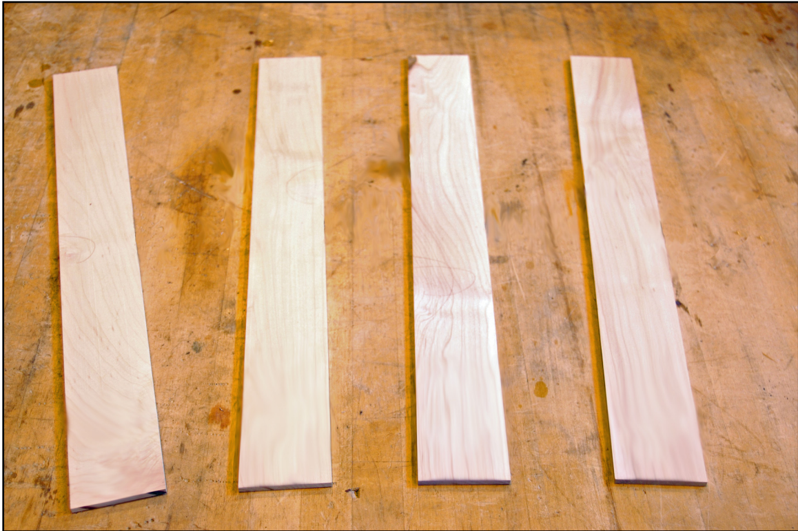
Figure 3.1 Completed maple specimens prior to thermocouple insertion. Very close inspection may reveal the pencil grader marks around defects; these were not specimens for bending. Photograph by author 2010.
