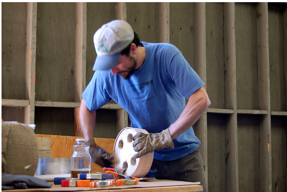
Figure 2.4 Galbreath attaches bent banjo hoop to cooling form. Photograph by author, 2008
