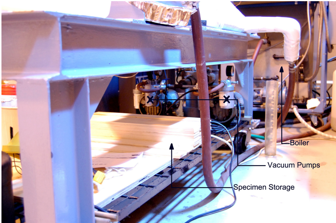
Figure 3.8 Lower shelf showing vacuum pumps indicated with “X”, boiler and specimen storage with “←”. Photograph by author 2010.
