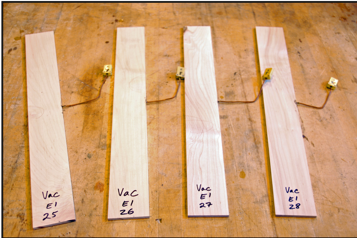
Figure 4.2 Specimens for Research Hypothesis #1 showing thermocouple placement Photograph by author 2010.
