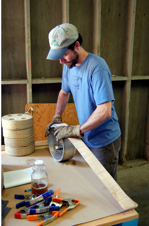
Figure 2.3 Greg Galbreath, luthier and “Buckeye Banjos” owner bends steamed curly maple around hoop mould. Photograph by author, 2008
