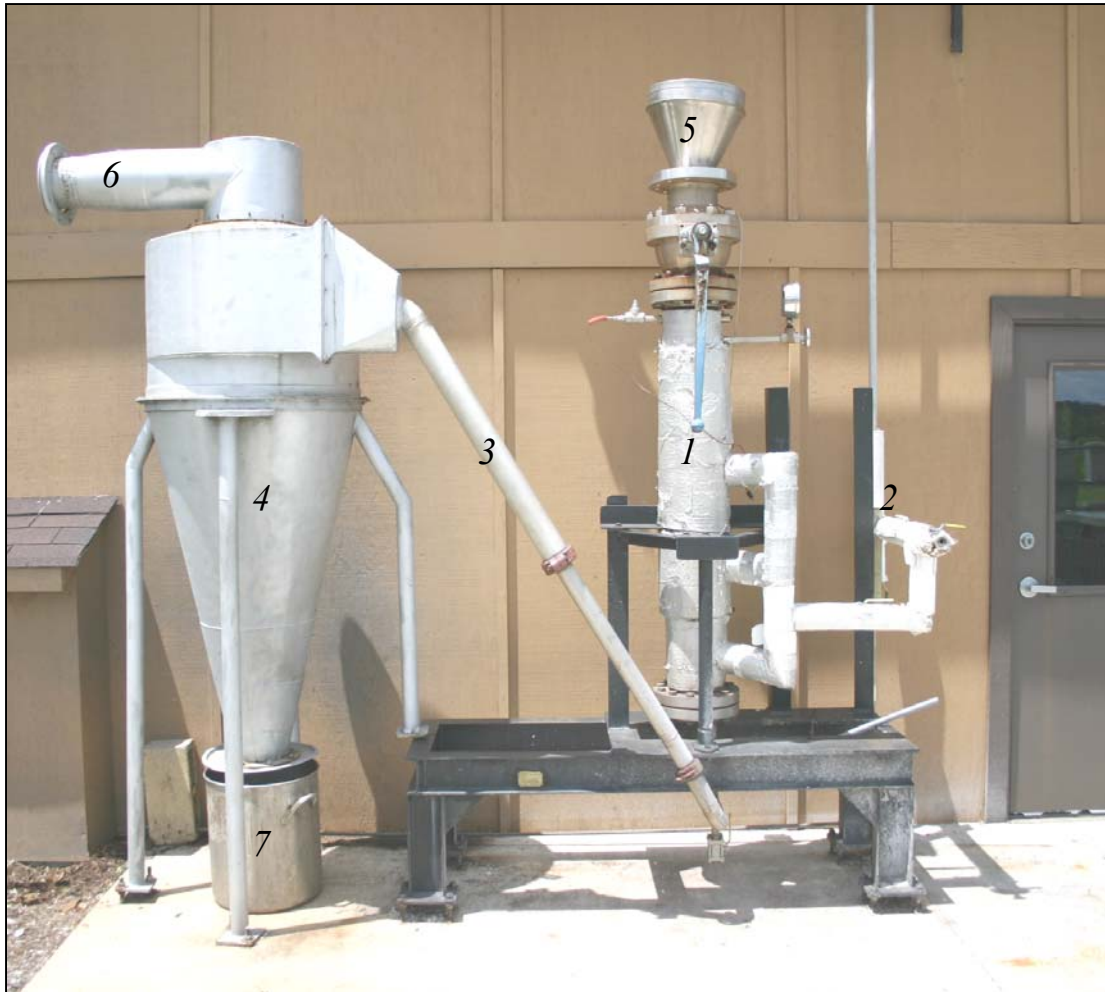
Figure 3.3 Steam explosion batch reactor
