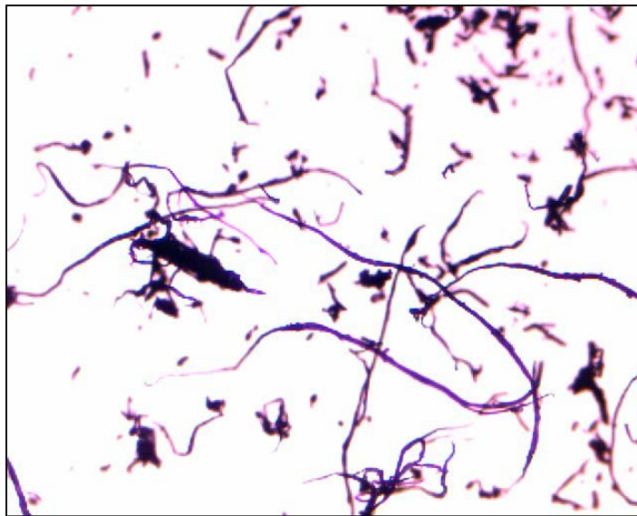
Figure 3.2 Optical microscope image of steam-exploded red oak fibers prior to wetlaying. Notice non uniformity in length and shape of fibers as well as presence of particles and fiber clumps. Magnification = 40x.
