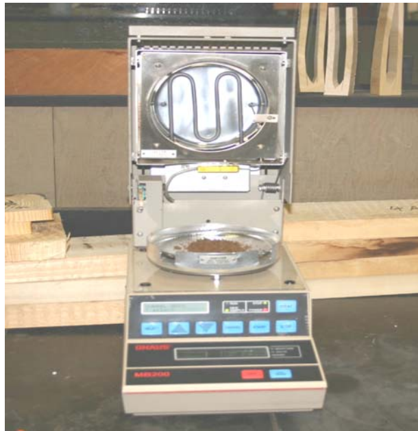
Figure 3.4 Ohaus MB 200 moisture balance
