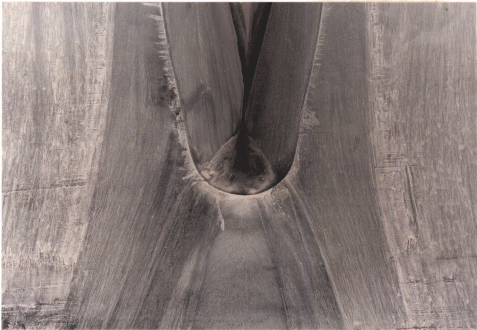
Figure 27. Photographs of the Nose Region (top), and Trailing Edge Region (bottom), Wing with Fillet at 0 Degrees Angle of Attack, Thick Boundary Layer, Boundary-Layer Tunnel.
