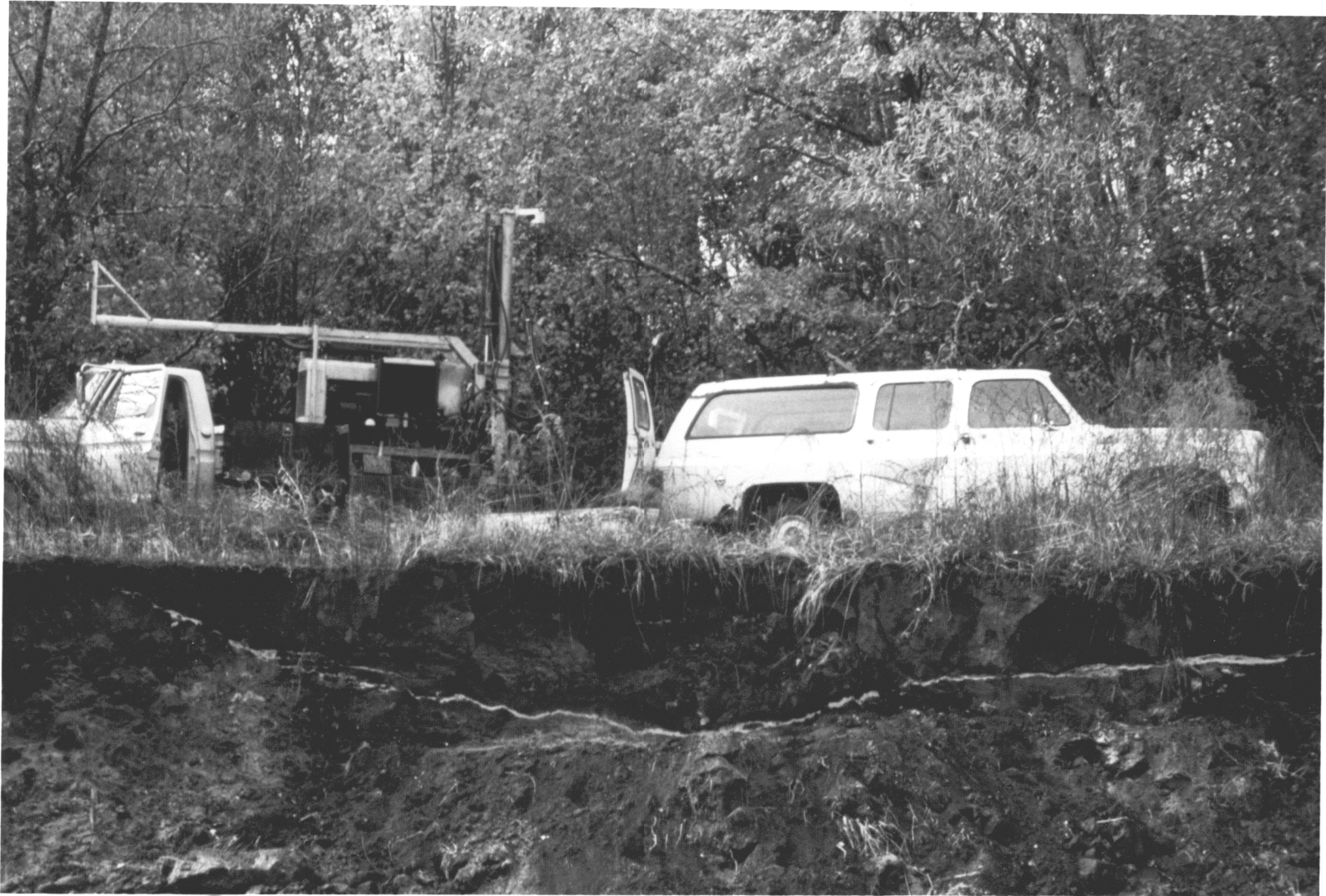
Figure 12. Cone Testing Operation at the Oakland Plantation Site. A thin white seam of vented sand can be seen in the wall of the sand pit.
