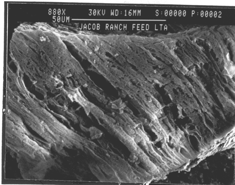
Figure 22. Electron Micrographs of Jacob's Ranch Wet-Screened Feed Coal: Above: 3 Siderite Inclusion - Below: 4 LT Ash Network (Fine Carbonates and Clay Lenses)
