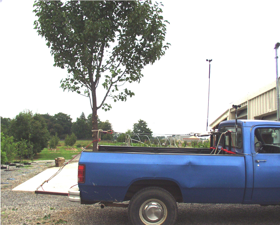
Figure 3: Completed assembly of tree, tree sled (in truck bed) and truck before the test began.
