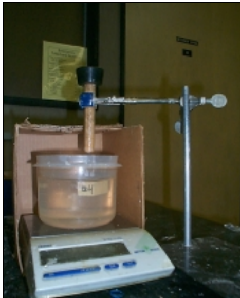
Figure 3.29: Specific gravity determination using water immersion method.
