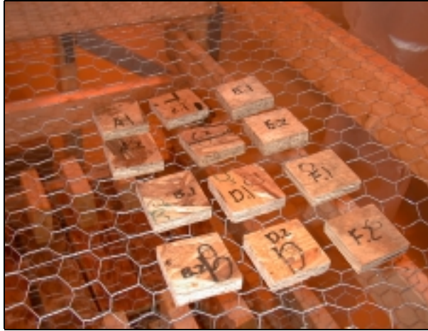
Figure 3.28: Representative side member samples positioned inside the climate chamber.
