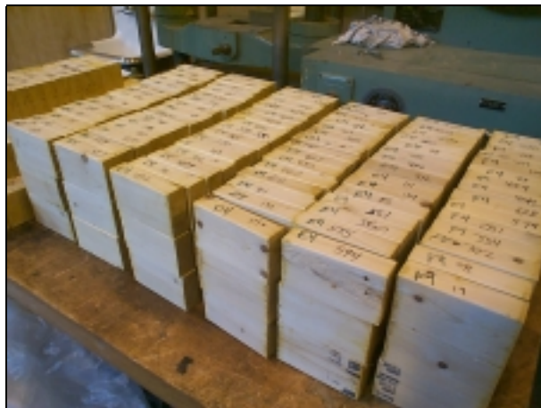
Figure 3.7: Main members with dry coat of Anchorseal ® end sealer.
