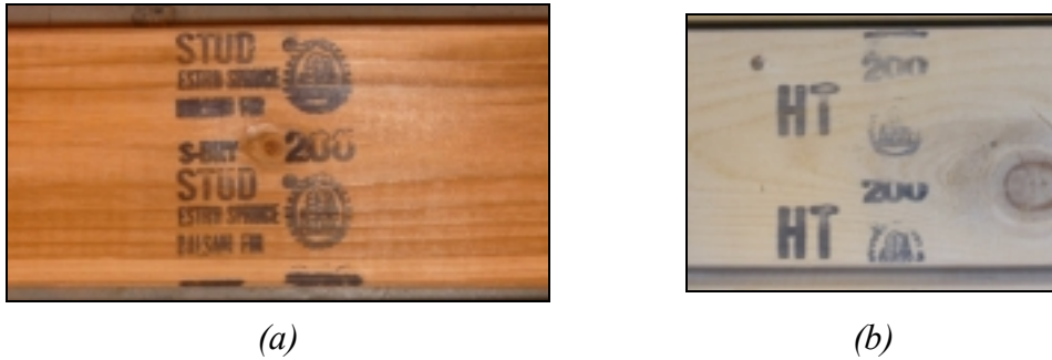
Figure 3.1: (a) Grade stamps and (b) heat treatment mark on main member materials.
