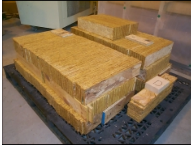
Figure 3.8: Side members with dry coat of Anchorseal ® end sealer.
