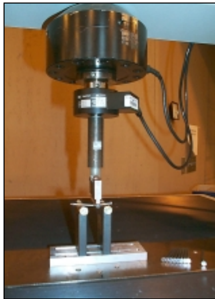
Figure 3.25: Fastener bending test.
