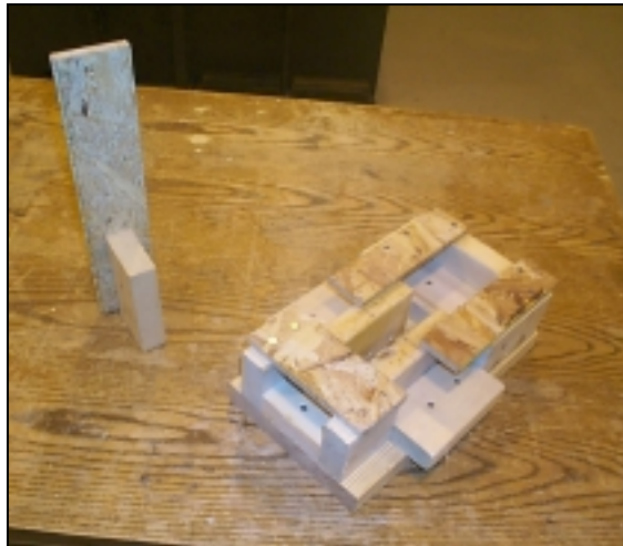
Figure 3.9: Connection specimen and nailing jig.
