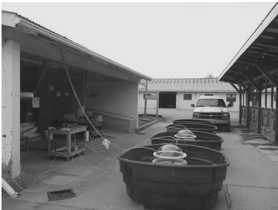
Figure 2-1. Manure storage experimental setup showing two tanks with flux chambers
