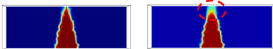
Figure 2: Conductive filament rupture by thermal diffusion
