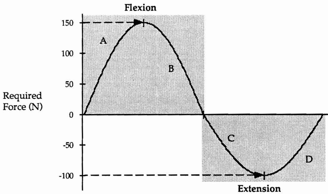
Figure 4.1 Characteristics of the track forcing function.
