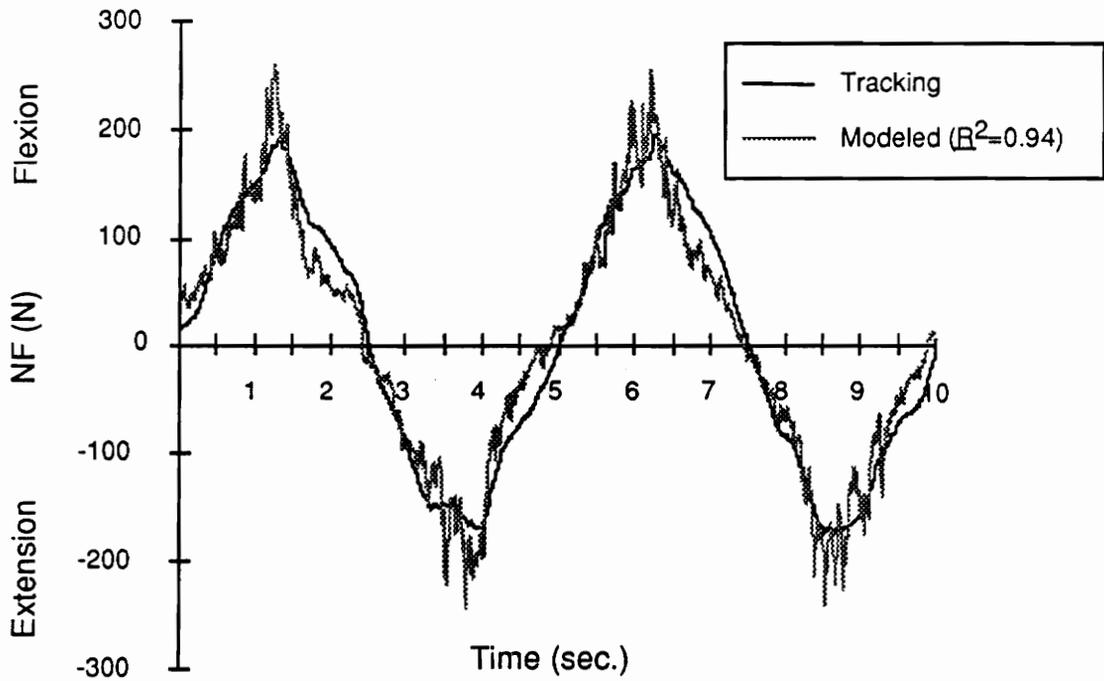
Figure 4.4 Data plot from a ten second sample sinusoidal tracking exertion (100% MVC, 0.2 Hz) showing isometric tracking force and modeled force.
