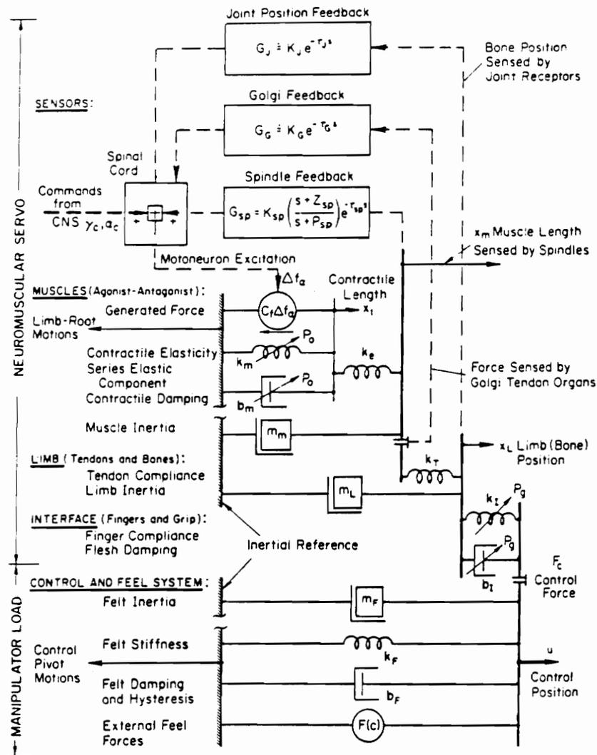
Figure 2.3 Second order differential control model of the neuromuscular control system (Jex, 1971).
