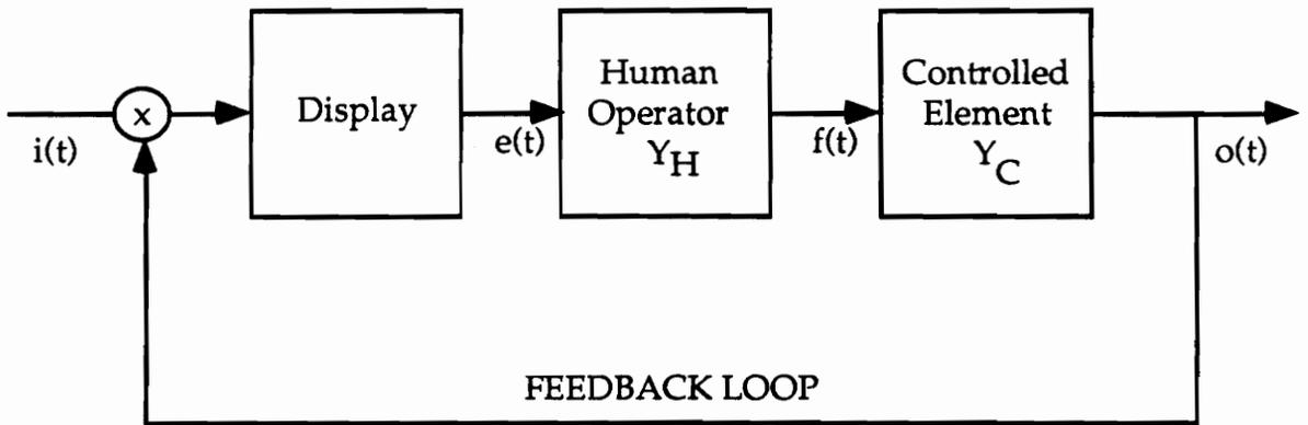
**Figure 2.2** Block diagram of compensatory tracking showing transfer elements (adapted from Wickens, 1984).
