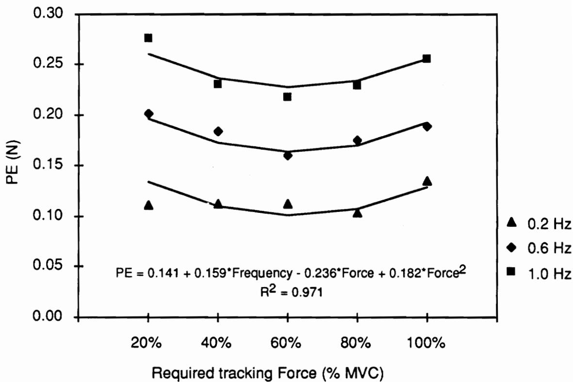
Figure 4.2 Two way interaction of Frequency and Force for proportional error and the polynomial regression model fit (solid lines).
