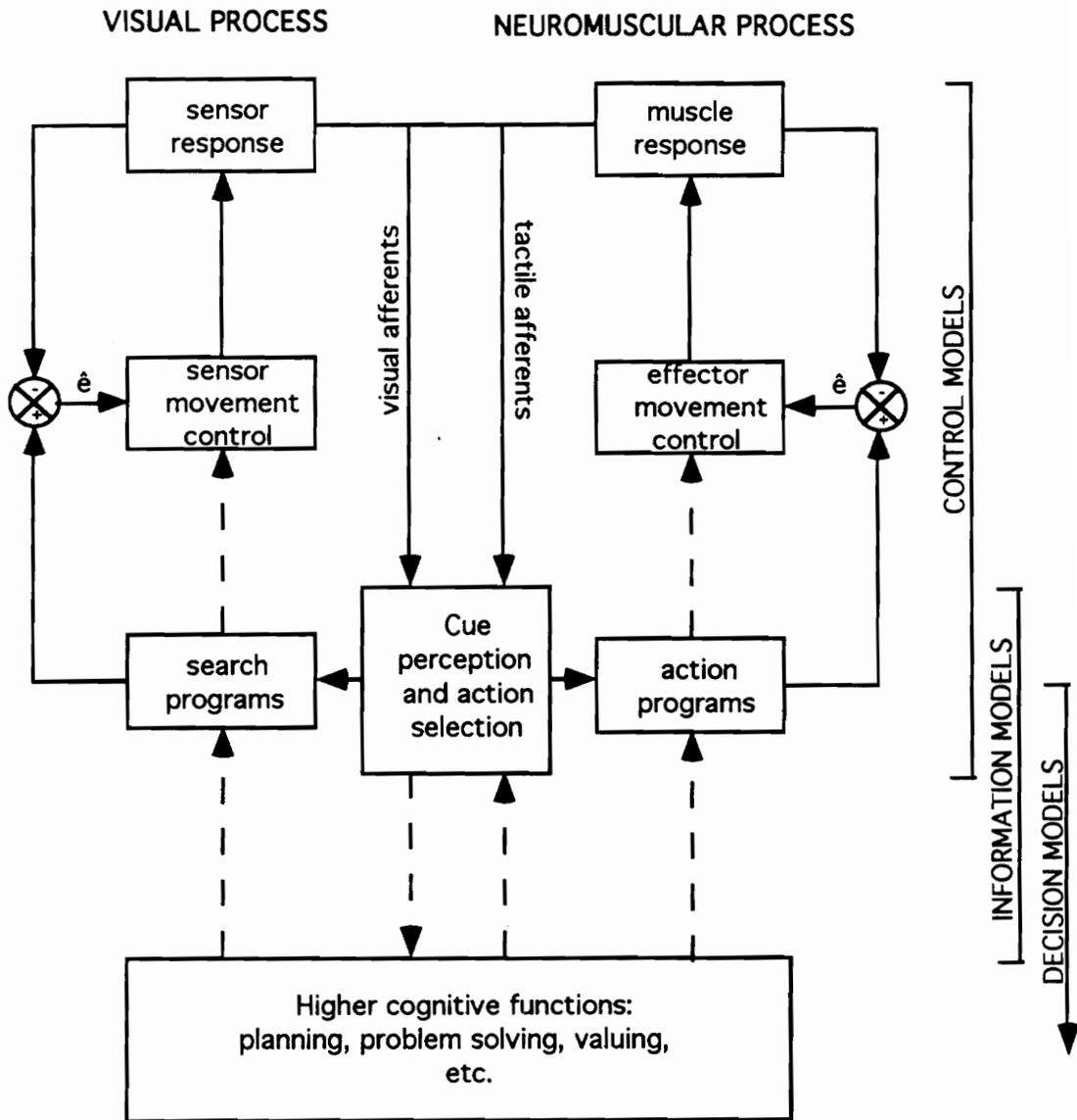
**Figure 2.1** Model of human movement (adapted from Sheridan and Ferrell, 1974).
