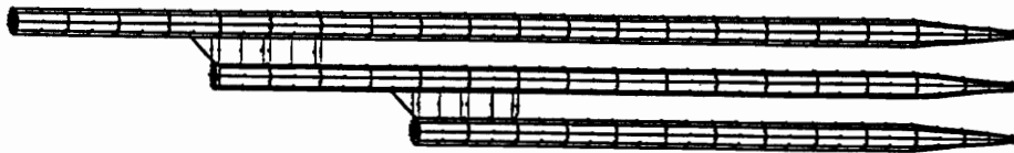
Figure 38. FEA stereocilia bundle model interconnected with few subapical bands. The number of subapical band elements was reduced from 21 to 11 elements to determine its effect on stiffness. This reduced stiffness by less than 1%.
