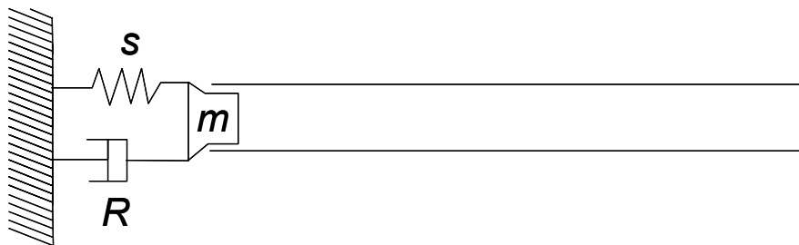
Figure 2.1. Schematic of the driver-cylindrical duct system where R , s , and m are the damping, stiffness, and mass of the driver respectively.
