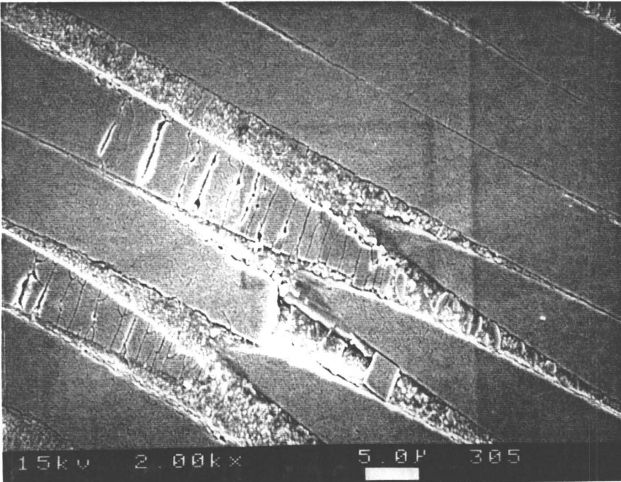
Fig. 43. (cont.) SEM's of wear scar in the anti-parallel orientation of graphite-epoxy. c) cracks in the fibers, fibers and matrix are seen to wear uniformly, d) transverse cracking and subsequent removal of the fibers.
