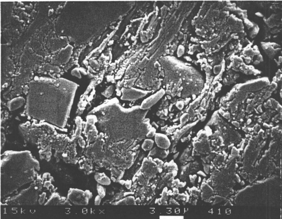
Fig. 62. (cont.) SEM's of wear scar in the normal orientation of carbon-PEEK. c) pieces of broken fibers in the wear debris, d) various sizes of wear debris.
