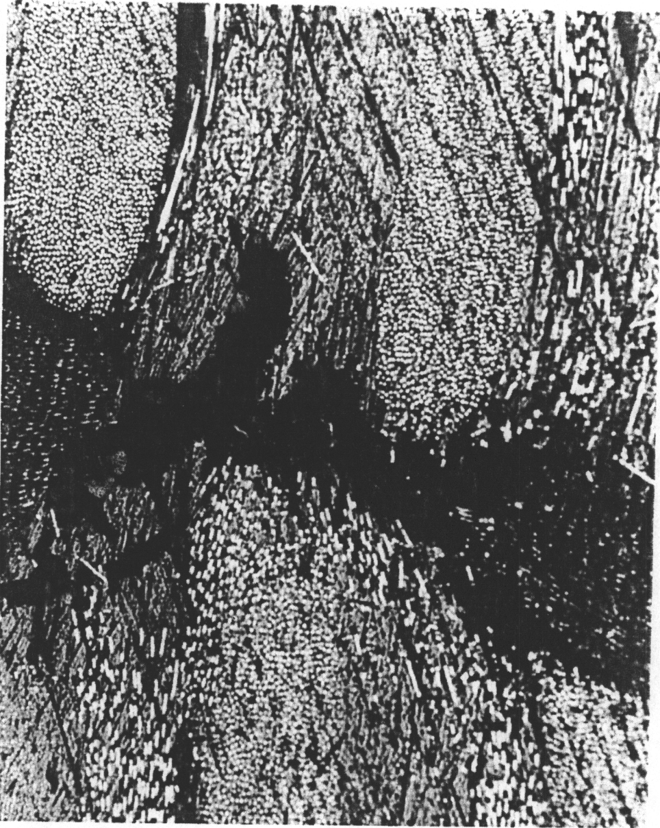
Figure 8. Layers Pulled Out-Of-Plane: 90° Specimen
