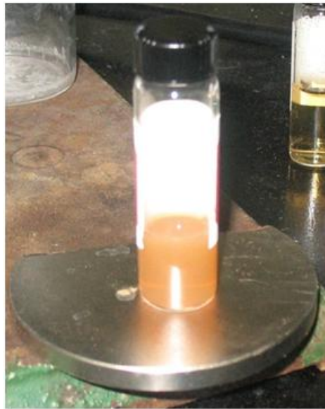
Figure 3.14. Magnetite clusters at Reynolds number of 5,000 under the influence of a magnetic field
