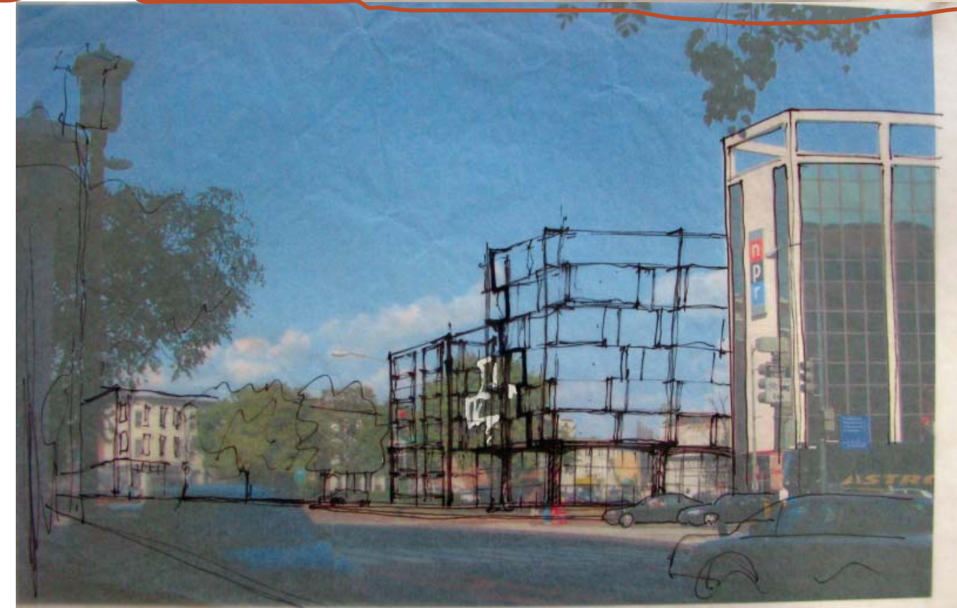
Study of juxtaposition of brick and steel facades to create a formal entry. Texture and scale on the vertical plane relate to the use of those textures on either side of the site.
